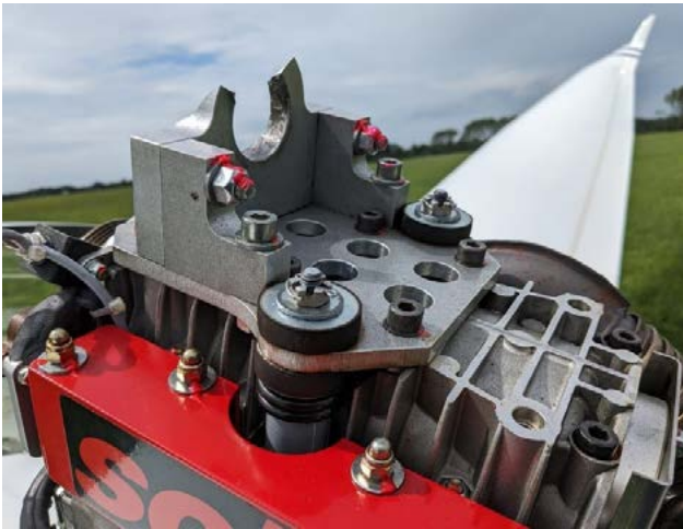
▲ The location at the engine where the hub was ripped off. (Source: gliding club)
