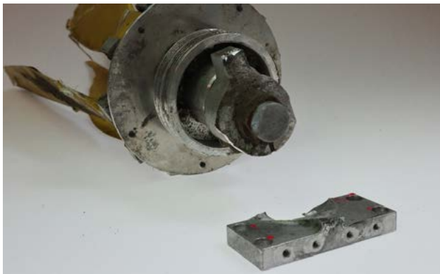
▲ The propeller with the fractured hub.
