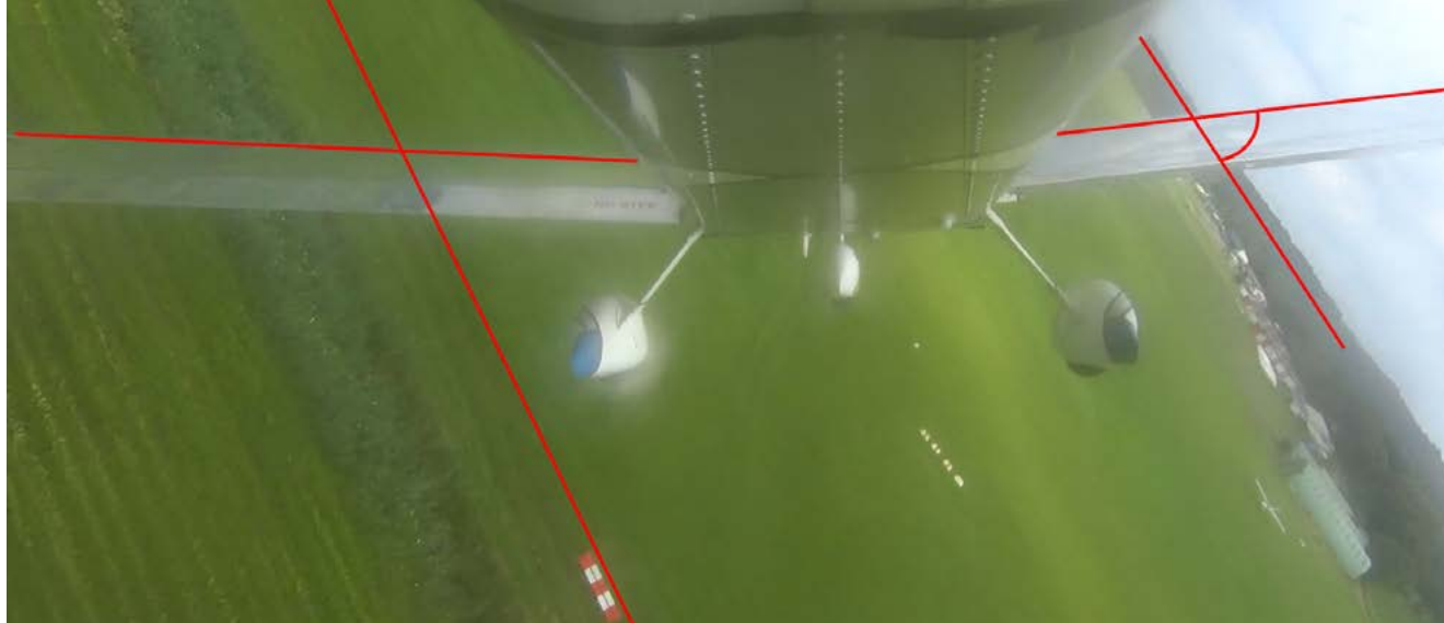
▲ Roll angle of about 70 degrees just before the crash. (Source: video camera underneath the tail (owner))
