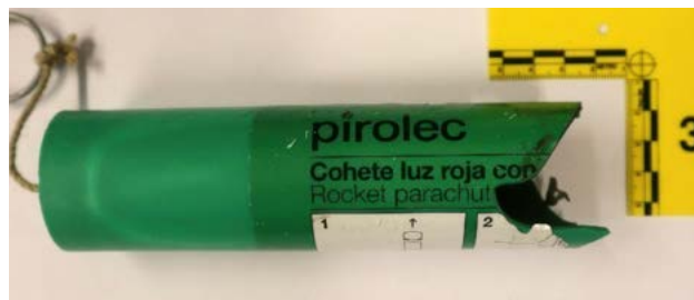
▼ Figure 10: Recovered remnants of the exploded flare. (Source: Bontekoning)
