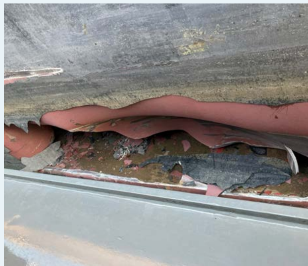
▲ Figure 28: Tear in the starboard side of the hull, 1 metre long and 50 centimetres wide. (Source: Union Shipping)
