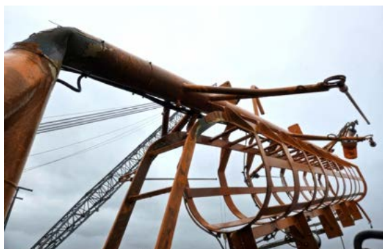
▲ Figure 29: Damage to the mast of the Eems Warrior. (Source: Amasus Shipping)
