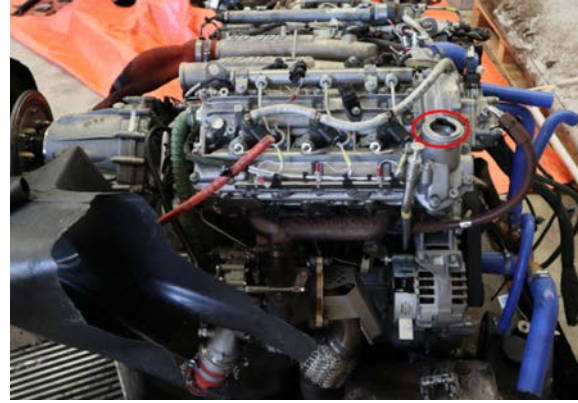
▲ Figure 8: Missing oil filler cap
