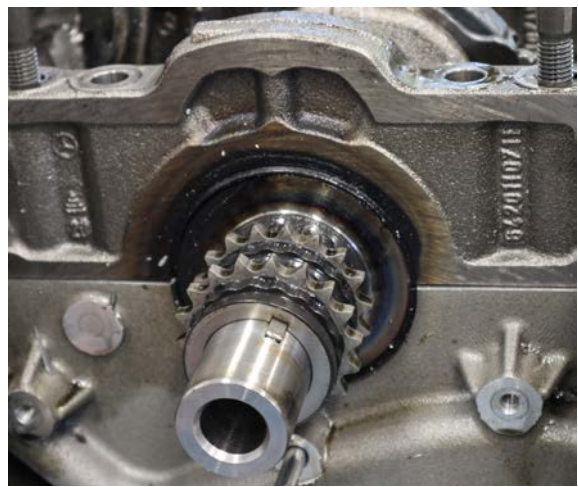
▲ Figure 12: Main #1 bearing heat imprint
