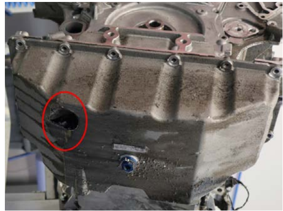
▲ Figure 10: Hole in oil pan
