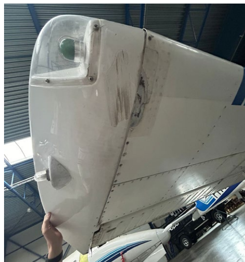
▲ The damaged wing tip. (Source: flying school)
