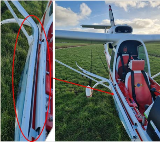
▲ Figure 1: The aircraft after the emergency landing. A small part of the canopy was still attached to the aircraft by means of the hinge.
