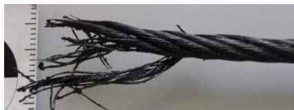
▲ A part of the broken cable.
