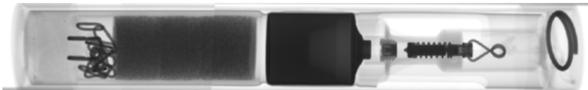
▲ Figure 6: X-ray photo (taken on Tahiti) of one of the flares from batch 113. (Source: Gendarmerie France)
