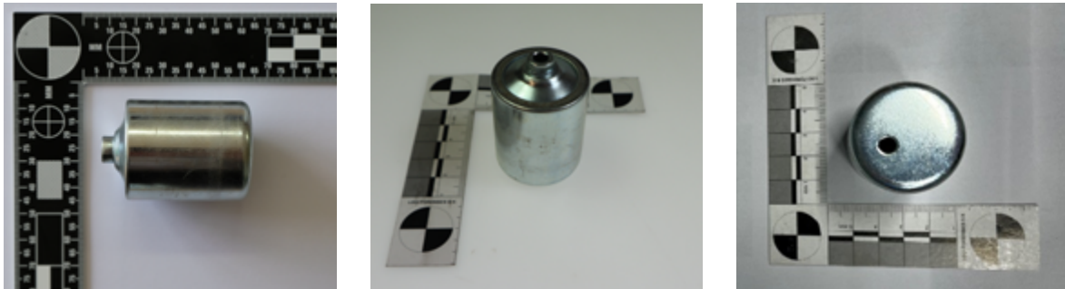
▲ Figure 7:1 (left): The motor, side view after sealing (hemming) lid.
