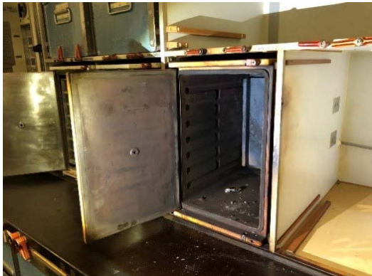
▲ The failed oven.
