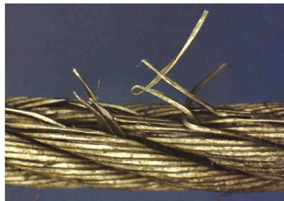
▲ Figure 9: Broken cable at position 832 cm from the reference position. (Source: Laboratory)
