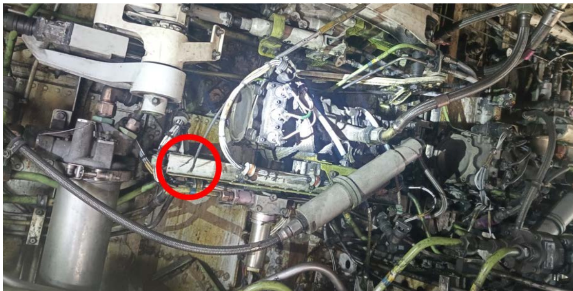
▲ Figure 1: One side of the broken aileron control cable, see circle. (Source: local ground engineer at Athens)
