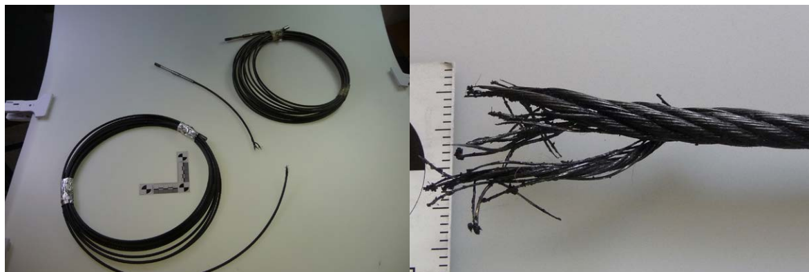
▲ Figure 6: Left, the two cables to be examined in the laboratory; Right, one part of the failed cable in detail.
