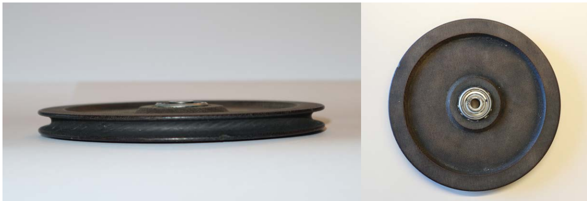
▲ Figure 10: The removed pulley located near the cable fracture.
