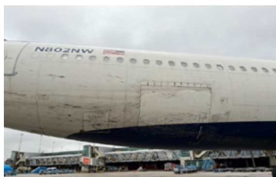
▲ Figure 4: Mud traces on the aft fuselage of the Airbus A330.
