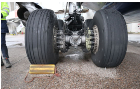
▲ Figure 3: Anti-rotation brake rod restraint cable. (Source: Operator)
