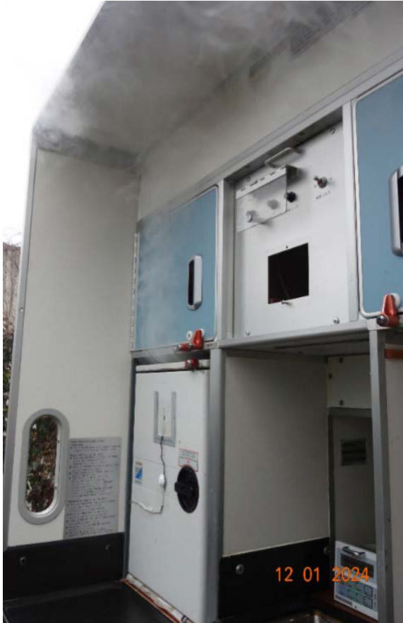
◀ Figure 7: Smoke coming from the oven in the test setup. (Source: B/E Aerospace)
