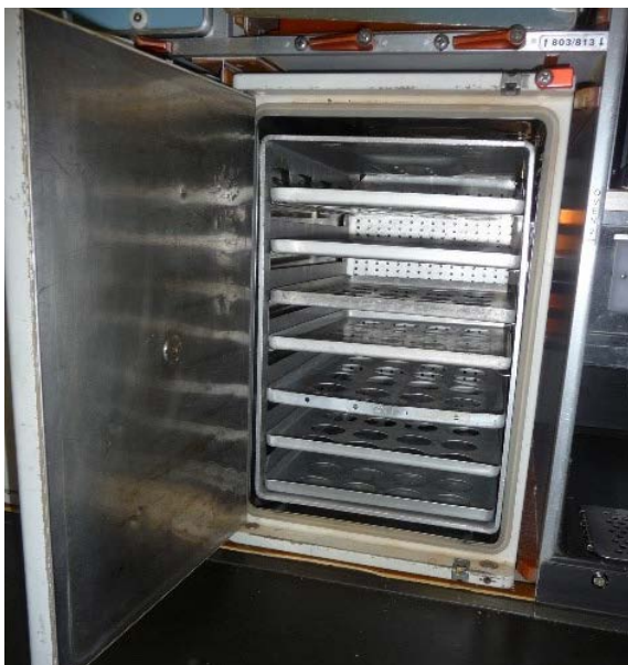
▲ Figure 3: Left, carrier with meal trays and mostly closed perforated backside in oven.
