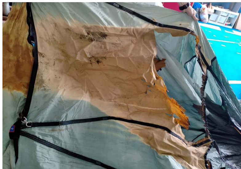
▲ Some burnt panels of the Cameron Balloons Ltd. Z-90. (Source: student balloonist)
