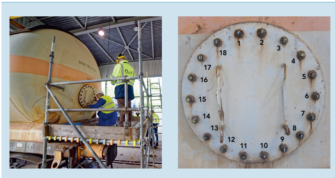
Figure 27: The left-hand photograph was taken during the inspection carried out on 06-05-2015 in Geleen. The right-hand photograph shows the numbering of the bolt connections on the manhole cover (1 to 18) for the purposes of reporting. (Photos: Dutch Safety Board)
