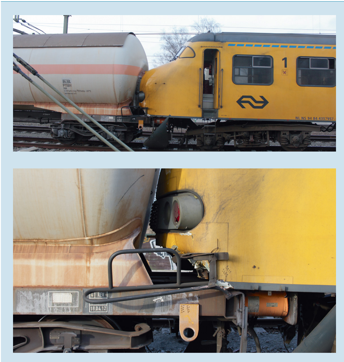
Figure 23: These photographs show that the nose of the passenger train had climbed up and over the buffers of the tank wagon, before colliding with the rear wall of the tank. (Photos: police)
