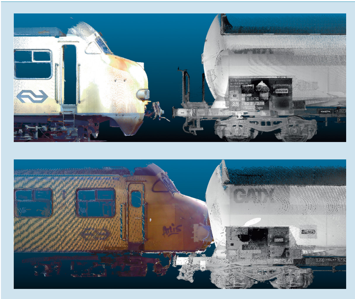
Figure 35: These pictures show the side views of the 3D scans of the passenger train and the tank wagon, in respect of one another. The top picture shows the undamaged fronts and the bottom picture the damaged fronts. (Photos: Dutch Safety Board - KLPD)
