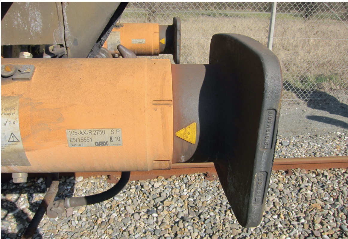
Figure 30: The crash buffers on the side of the tank wagon not run into showed no permanent deformation. (Photo: Dutch Safety Board)
