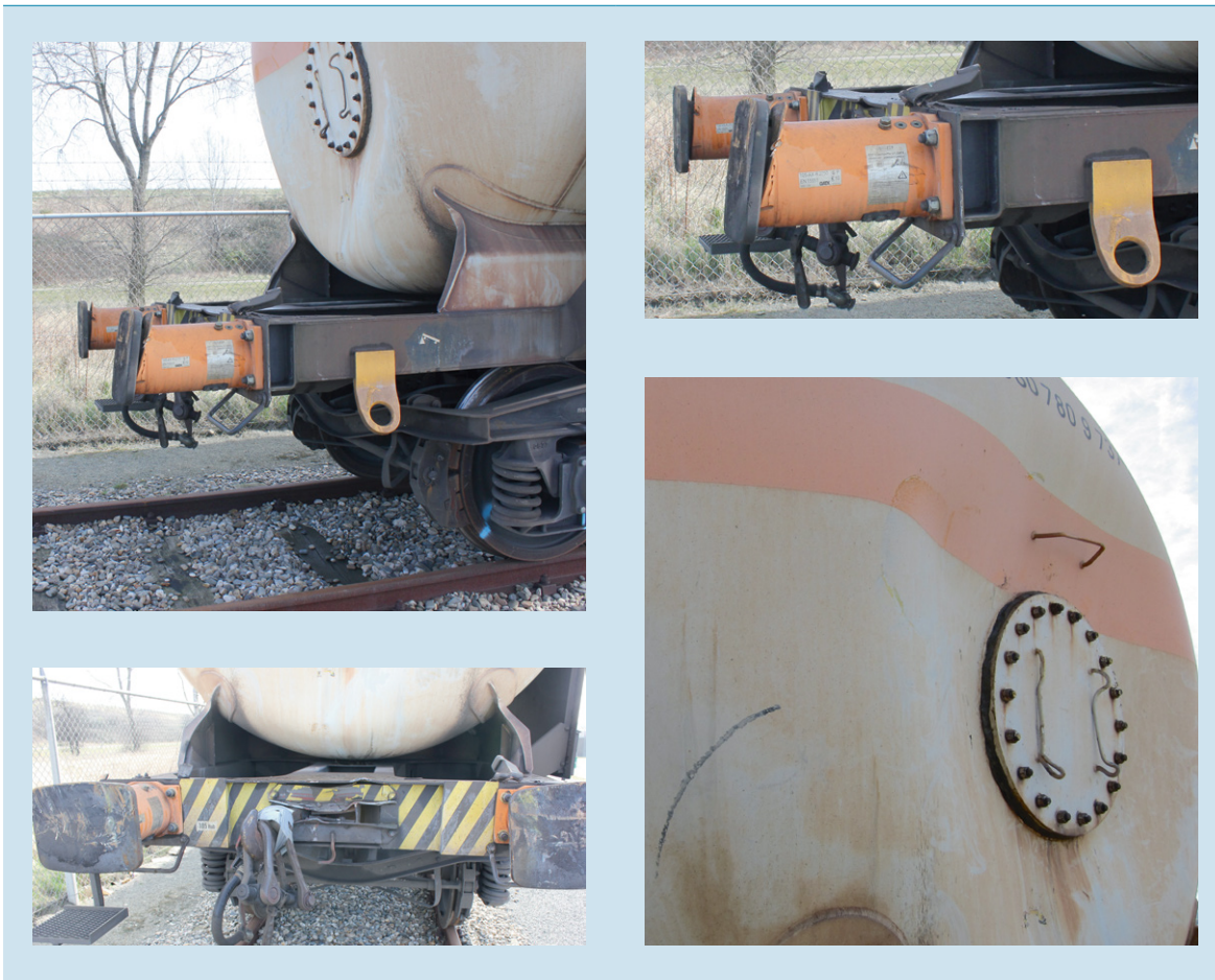
Figure 28: These photographs show the damage to the tank wagon. (Photos: Dutch Safety Board.)
