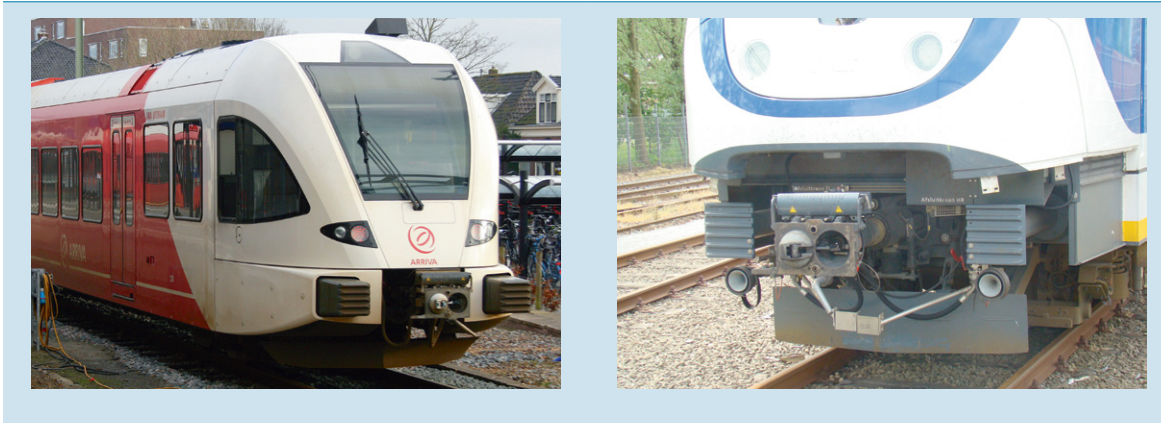
Figure 48: Both photographs show a modern passenger train equipped at the fronts with crash absorbers. On the train on the left-hand photo the crash absorbers are visible (on both sides of the automatic coupler). The right-hand photograph is a train of the type SLT operated by NS Reizigers: if the bottom section of the front panel is removed, the two crash absorbers and the obstacle deflector become visible. (Photos: left = Roel Hemkes, right = Dutch Safety Board)
