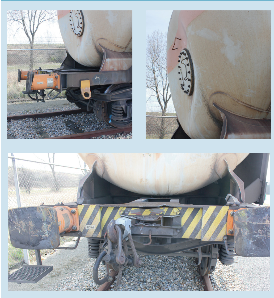
Figure 25: These photographs show the damage caused by the collision to (the back of) the rearmost tank wagon. (Photos: police)
