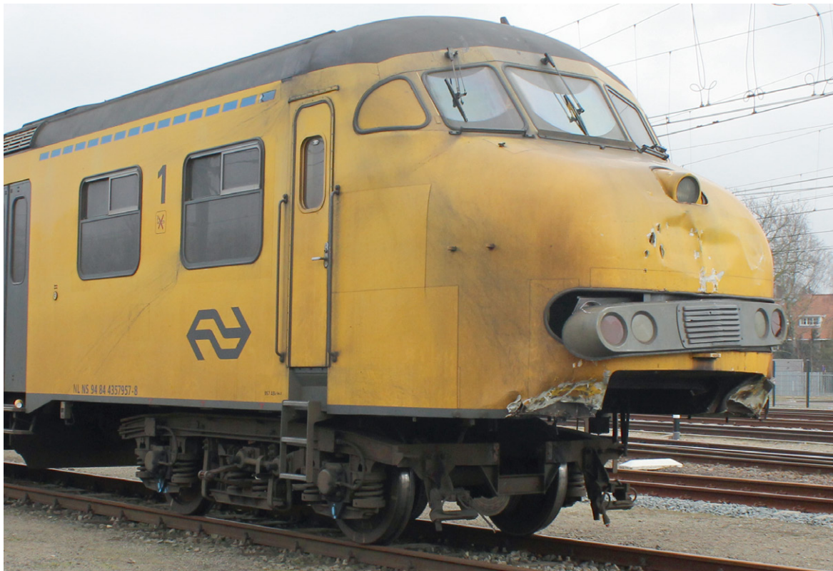
Figure 47: This photograph shows the damage to the front of the passenger train (Mat'64) involved in the accident in Tilburg. When the photograph was taken, the automatic coupler, which was seriously deformed, had already been removed. (Photo: police)
