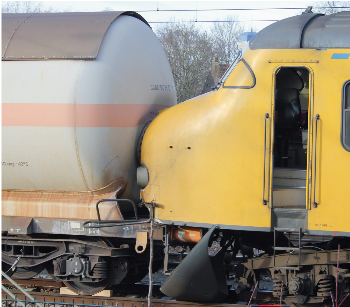
Figure 6: The front of the passenger train rose up and over the crash buffers on the tank wagon, and ended up against the tank. (Photo: Dutch Safety Board)
