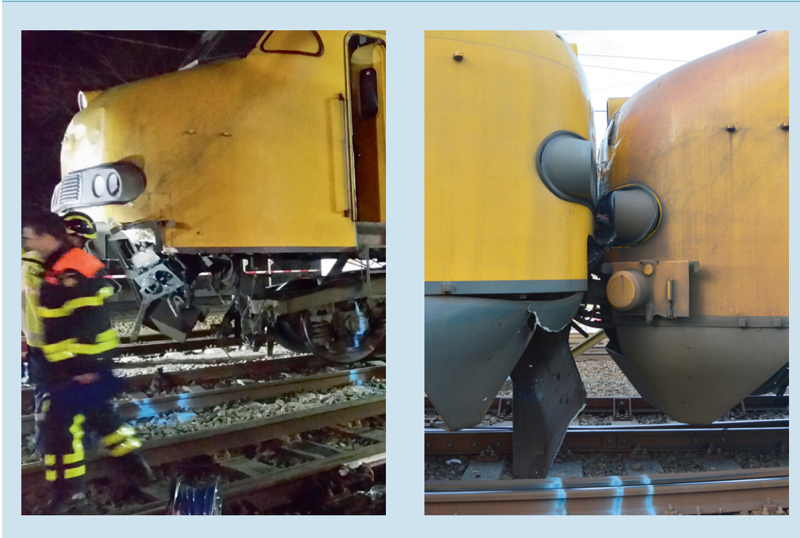
Figure 24: These photographs show the damage to the passenger train. The left-hand photograph shows the front end of the front multiple unit, the right-hand photograph shows the connection between the two multiple units. (Photos: left = fire brigade, right = police)
