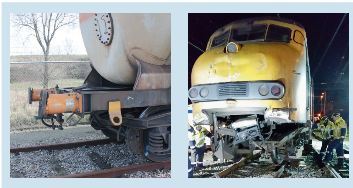
Figure 7: The damage to the rear of the tank wagon (left) and the front of the passenger train (right). (Photos: left = Dutch Safety Board, right = fire brigade)
