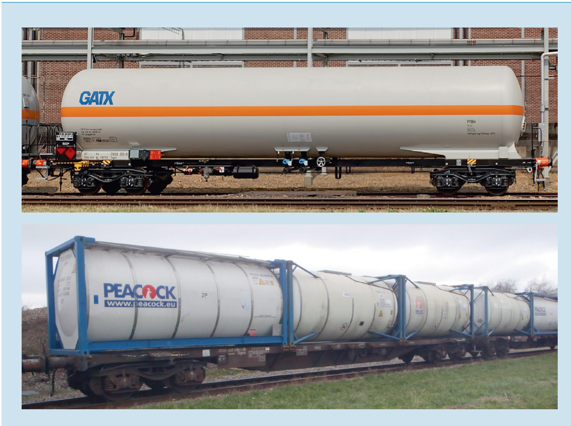
Figure 11: Examples of a tank wagon (top) and of three tank containers on a container carrier wagon (below). (Photos: SABIC)
