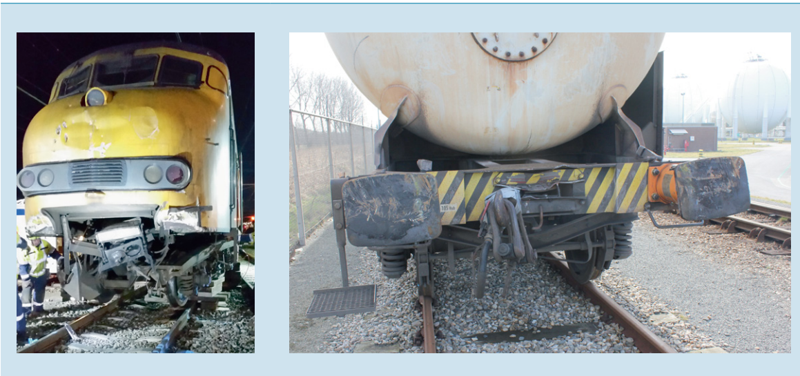
Figure 36: These photographs show the damage caused by the collision on the front of the passenger train (left) and the back of the tank wagon (right). On the front of the passenger train we see the impressions of the buffers and the manhole cover of the tank wagon; on the top section of the buffers of the tank wagon, we see an impression of the passenger train. (Photos: left = fire brigade, right = Dutch Safety Board)
