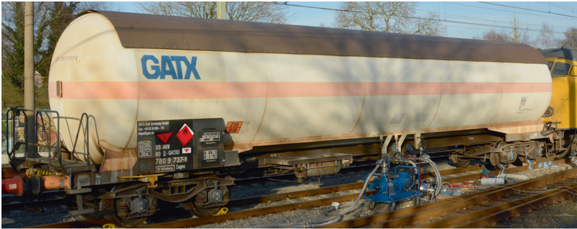
Figure 10: The damaged tank wagon was pumped empty with mobile pumps. (Photo: Dutch Safety Board)
