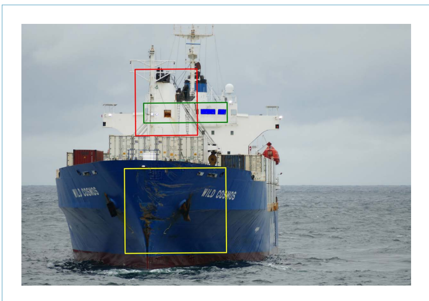
Figure 11: This picture shows that the starboard windows in the green rectangle are blocked by the cranes in the red rectangle. (Source: Danish Fisheries Inspection)
