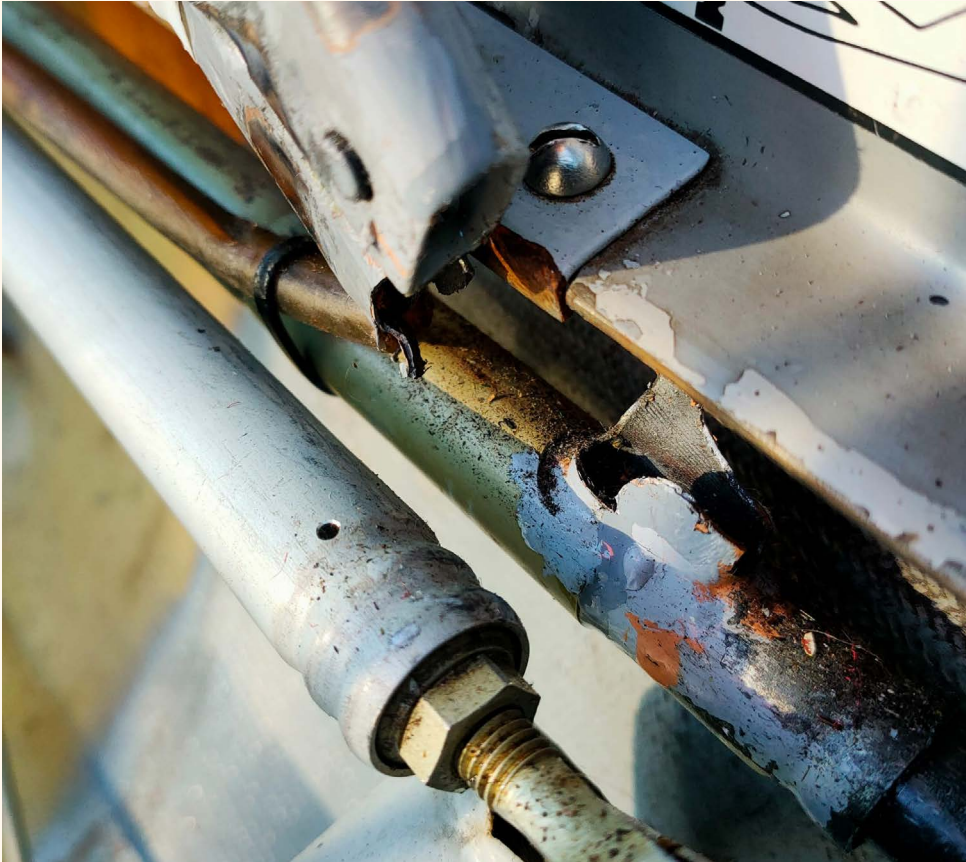
◀ The broken airbrake lever. (Source photograph on the left: gliding club)
