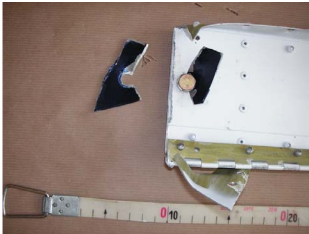
Figure 13: failed right wing rear spar attachment assembly.
