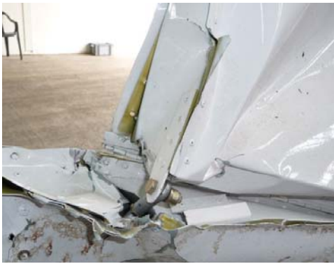
Figure 10: damage to the right aileron drive (inboard- and outboard side)
