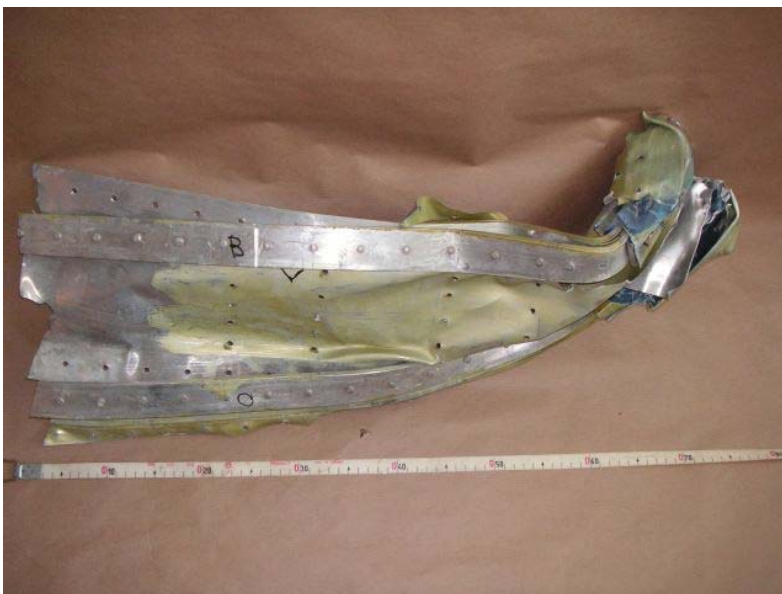
Figure 8: removed part of right wing main spar
