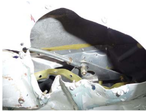
Figure 10: damage to the right aileron drive (inboard- and outboard side)
