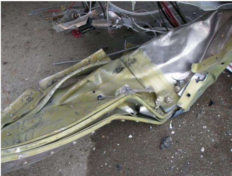
Figure 7: buckled right wing main spar
