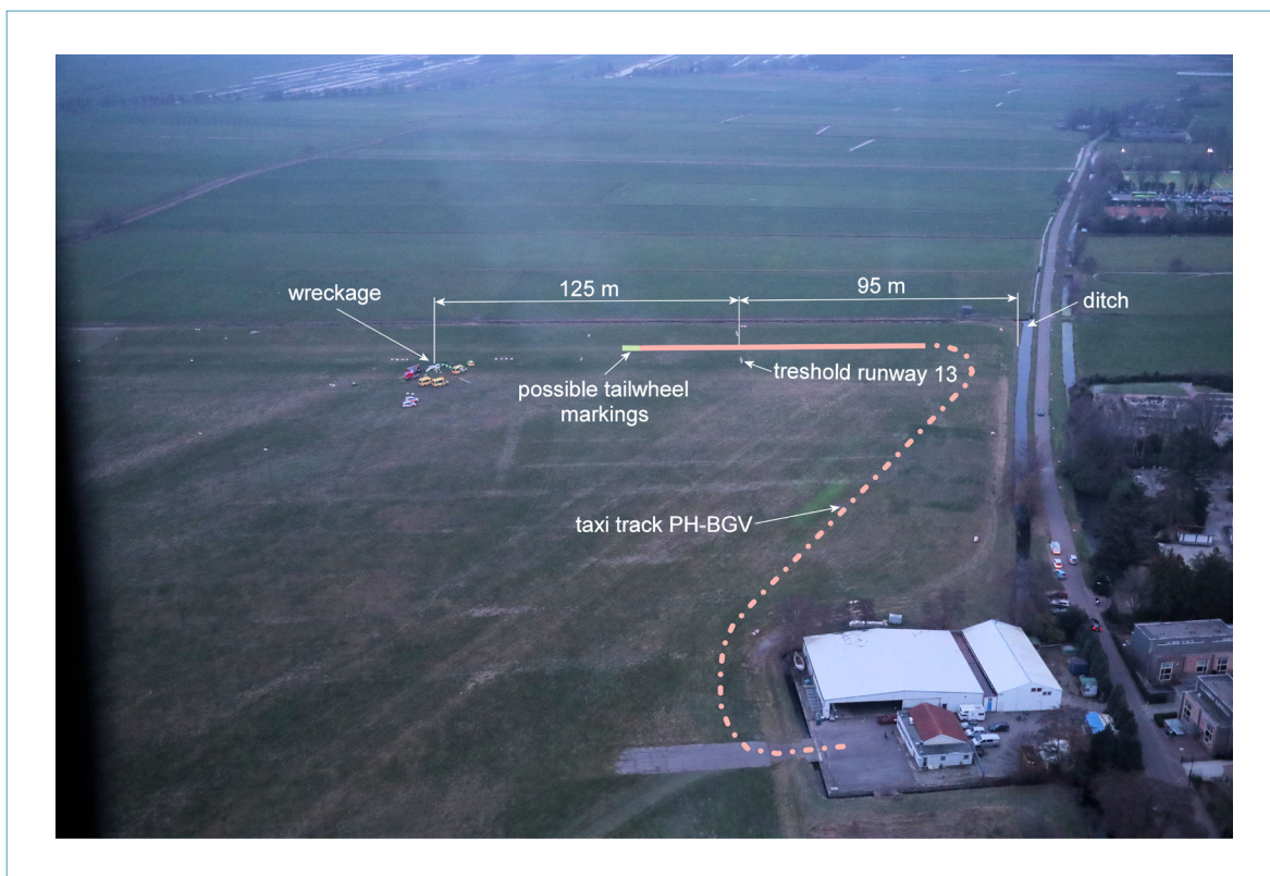
Figure 2: Overview of taxi route and take-off dimensions. (Source picture: Dutch Aviation Police)
