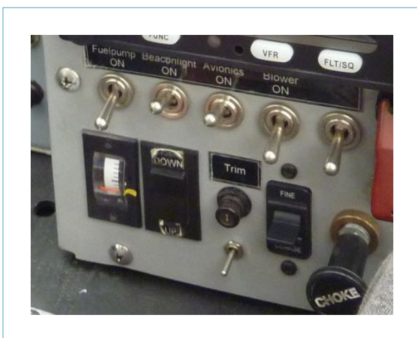
Figure 4: The trim indicator with yellow bug during flight a few years before the accident.
