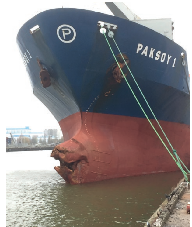
Damage to the bulbous bow of the Paksoy 1. (Source: Dutch Safety Board)
