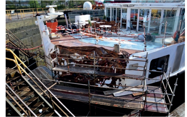
Damage to the river cruise ship. (Source: Dutch Safety Board)
