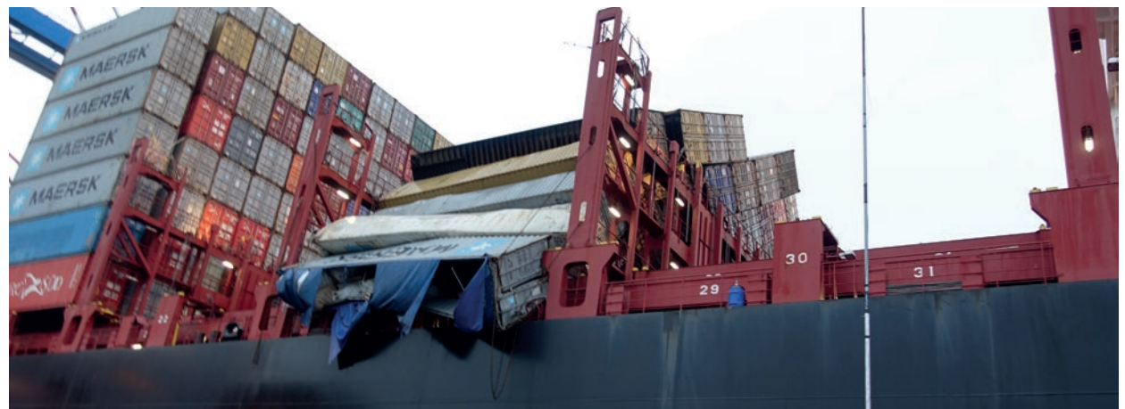
Containers hanging overboard. (Source: Dutch Safety Board)
