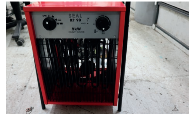
9 Kw electric heater. (Source: Dutch Safety Board)
