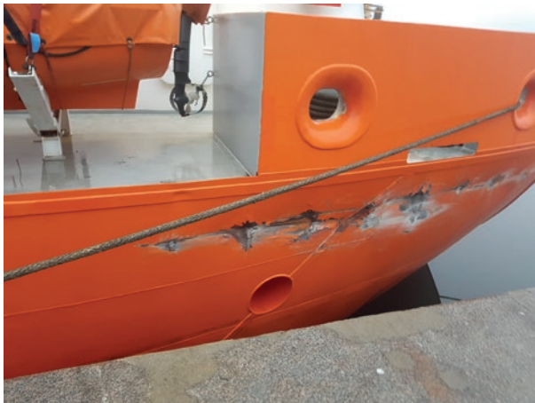
Damage following collision with the quayside. (Source: Ship operator)
