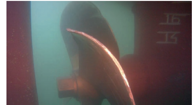
Damage to propeller blade. (Source: Ship operator)
