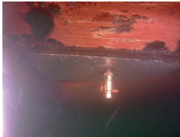
Temporary repair to ship's skin. (Source: Ship operator)
