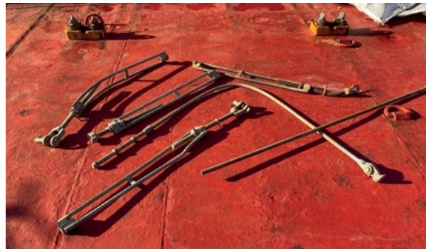
Damaged lashing equipment after the loss of containers.
