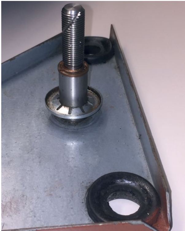
Inverted safety cover with venting bolt. (Source: Dutch Safety Board)
