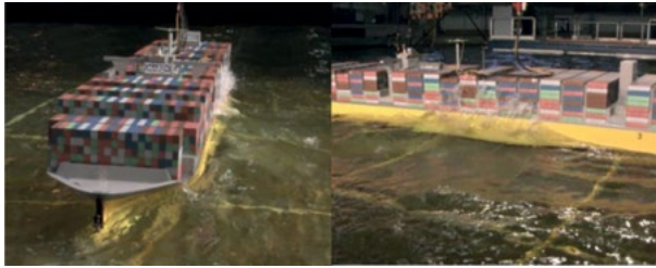
Observation of green water during de basin tests by MARIN.
