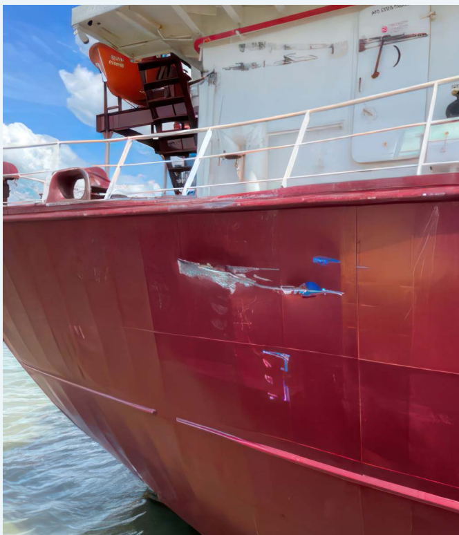
▲ Damage Oralora. (Source: DMAIB)
