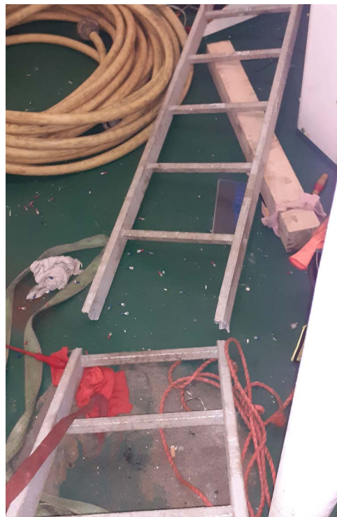
▲ The broken ladder on board the Arklow Brave. (Source: Arklow)
