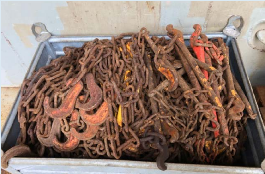
Figure 19: A container with lashing chains and tensioners on board the vessel.
