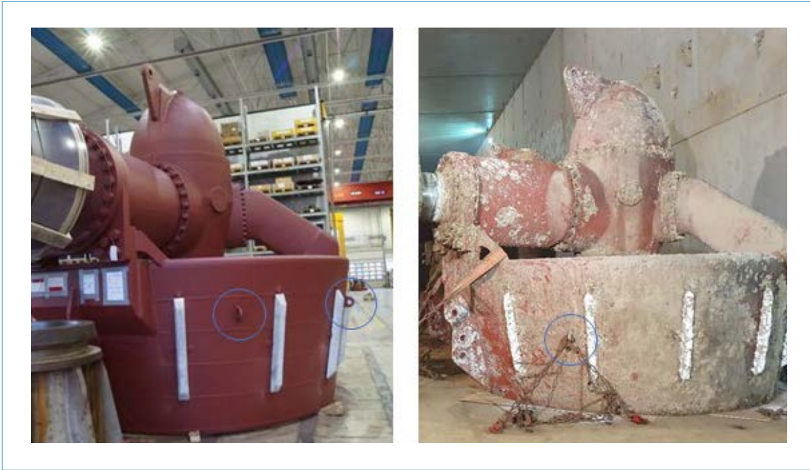
Figure 13: The photo on the left is the one provided by the freight broker and shows an azimuth thruster with two padeyes. The photo on the right shows one padeye on one of the azimuth thrusters in the hold. Note that the position of the padeye differs from the position of the padeye in the photo on the left. (Source: Amasus)
