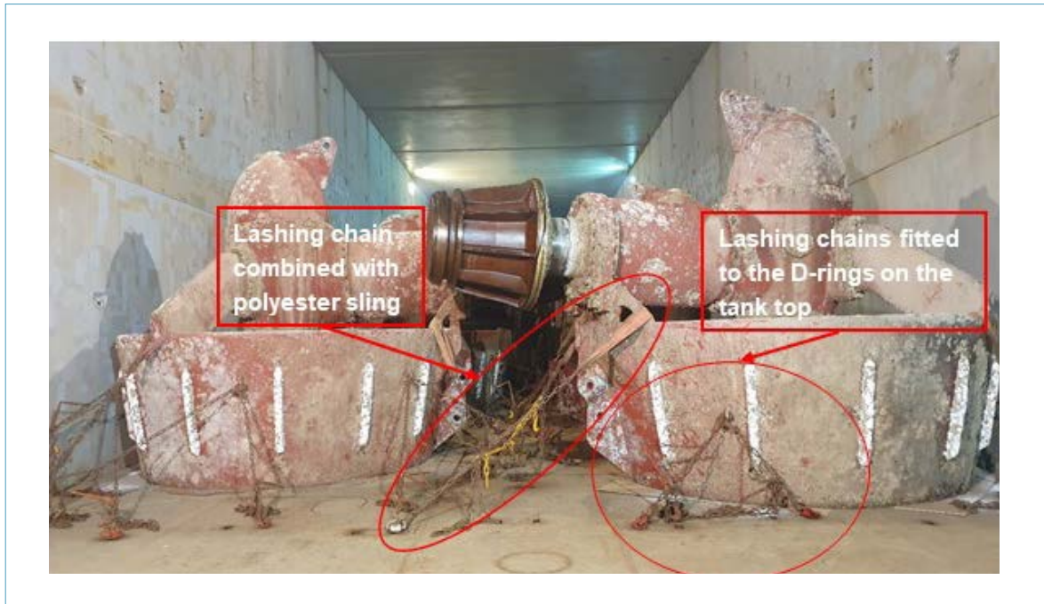
Figure 4: The thrusters as they were stowed in the hold, showing the lashings. Photo taken from the front of the hold looking aft. (Source: Amasus)
