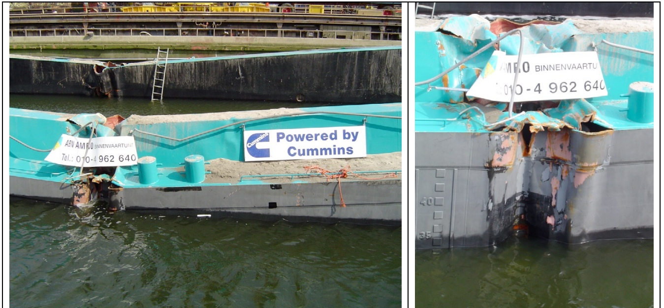
Figure 5 and 6: Photos of the sagging of the side of the ship
