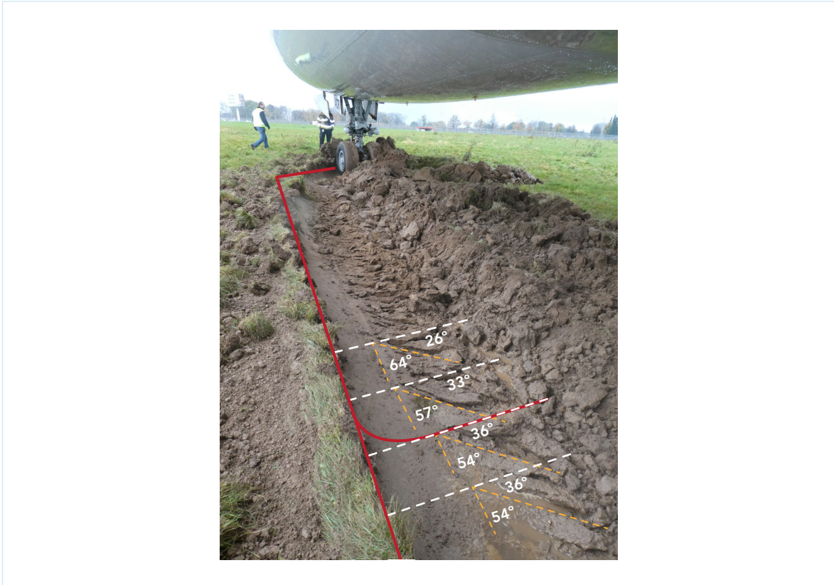
Figure 6: Analysis of the nose wheel track. The red line indicates the orientation of the aircraft; the yellow line indicates the angle of the nose wheel.
