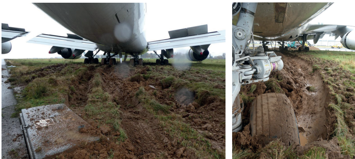
Figure 5: Photographs of wheel tracks in the soft ground.
