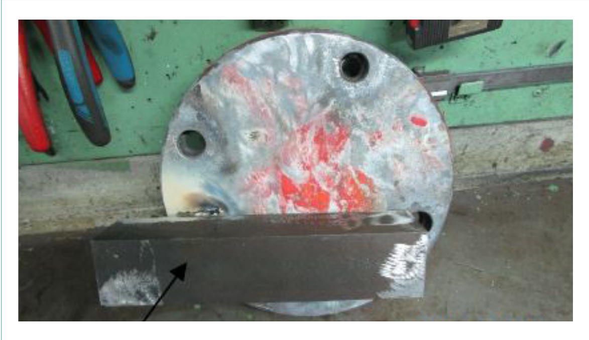
Figure 8: The cover plate onto which an angle bar is welded as a tool for removing the cover plate from the wheel. (Source: Holwerda Shipmanagement B.V.)
