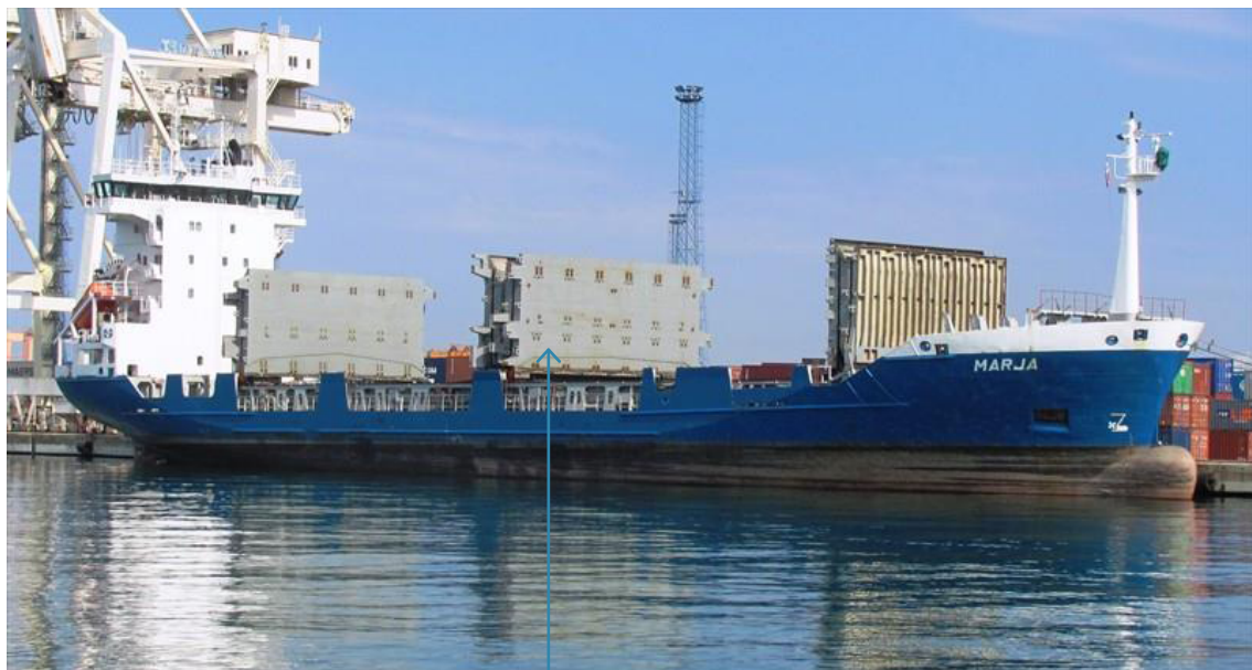
Hatch cover 2B, with behind it hatch cover 3A. Both in opened position.
