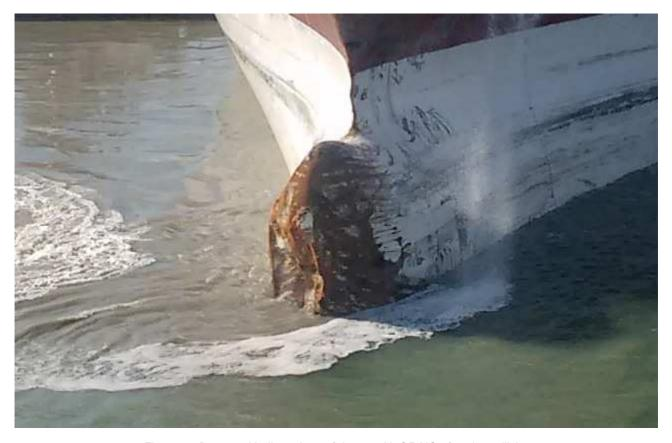
Figure 9 - Damaged bulbous bow of the mts AL ORAIQ after the collision
