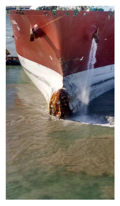
Figure 4 - Damage to the mts AL ORAIQ after the collision
