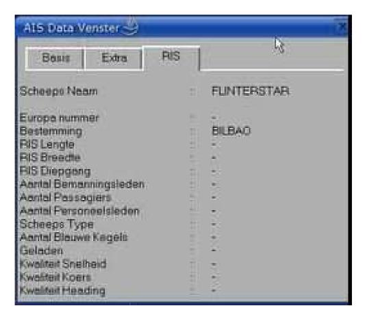
Figure 7 - Detailed Automatic Identification System data from mv FLINTERSTAR not filled out
