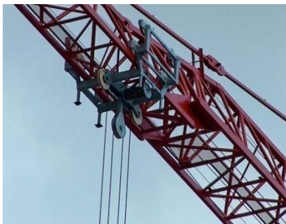
Figure 3 Crane trolley with double drive system
