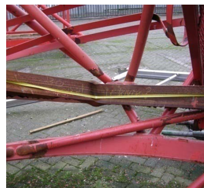
Figure 10 – Bent mast sections Figure 11 – Broken connecting part Figure 12 – Buckled tower leg (Photograph: Aboma Keboma).
