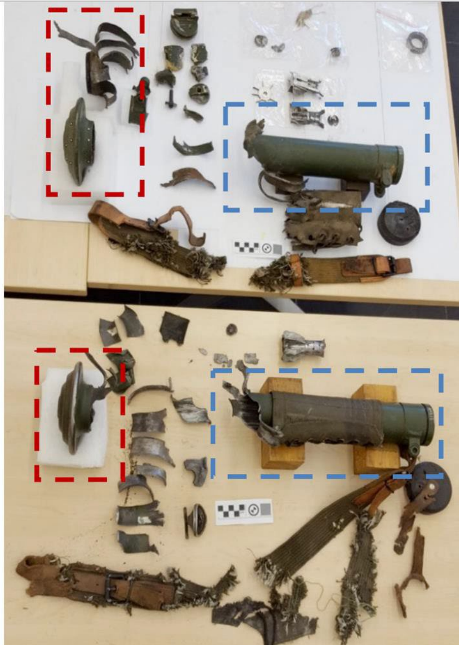
Figure 26: Damage to the mortar tube from the accident (top) and after the test with the fuze in armed position by KC W&M (bottom). The picture contrasts the length of 'petaling' of the tube remnants near the base plate (red boxes) and the lengths of the residual tube from the muzzle end (blue boxes). (Picture: TNO)
