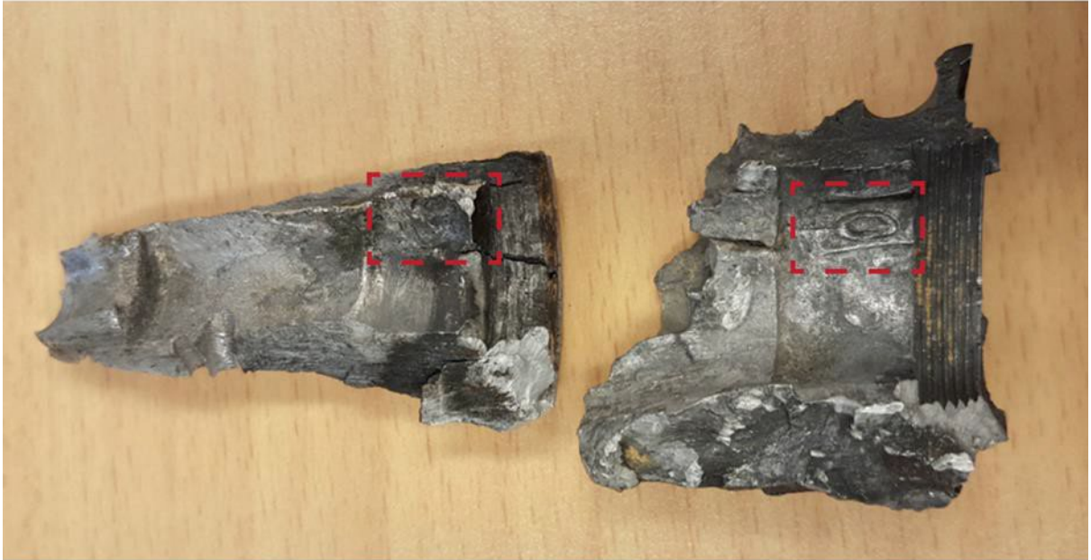
Figure 27: Imprint of the slider and slider spring on the inner wall of the fuze body from the test in armed position (left) and on the inner wall of the fuze body from the accident mortar round (right). (Picture: TNO)
