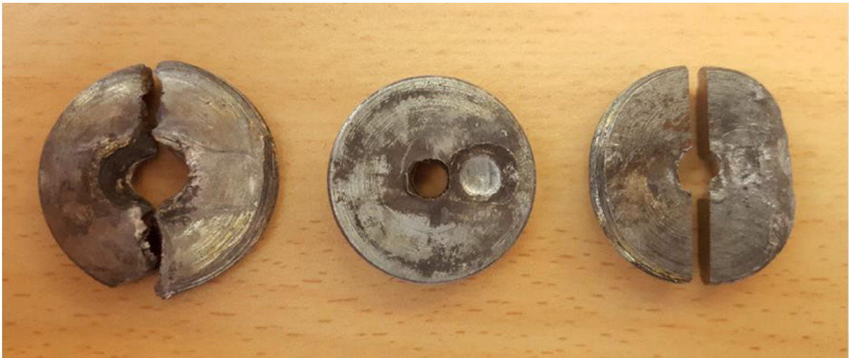
Figure 30: Top surfaces of the explosive train interrupter plate from the test in armed position (left), from the test in safe position (centre) and from the accident (right). The plate from the test in armed position is broken as a result of the detonation, the plate from the accident was recovered in one piece, but cut in half for further examination. The off-centre dent in the accident plate is thought to demonstrate the detonator fired in the 'safe' position. (Picture: TNO)
