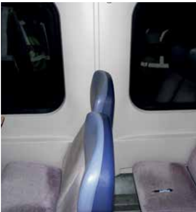
Figure 10: Top: damaged ends of coaches. Bottom left: deformed seat. Bottom right: damaged seat. Source: Dutch Safety Board
