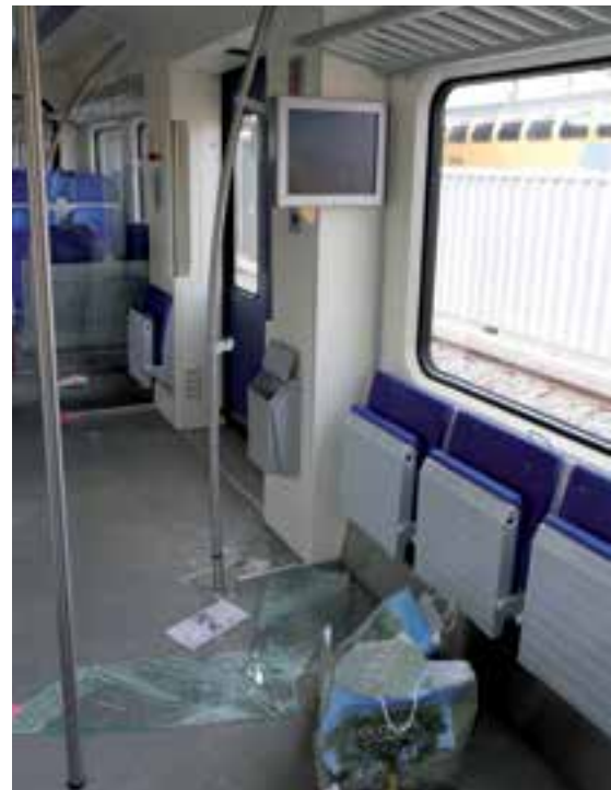
Figure 21: Glass damage. Top left: entrance to intercity passenger compartment; Top right: broken glass partition wall in sprinter; Bottom left: shattered glass door in sprinter; Bottom right: broken and dislodged glass shards in sprinter. Source: Dutch Safety Board
