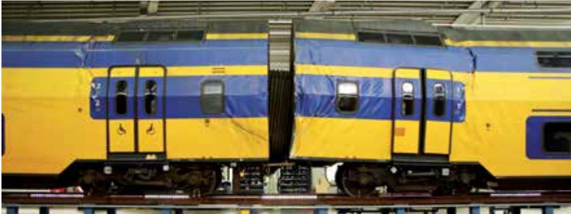
Figure 16: Deformation of the ends of the intercity coaches. Source: Dutch Safety Board
