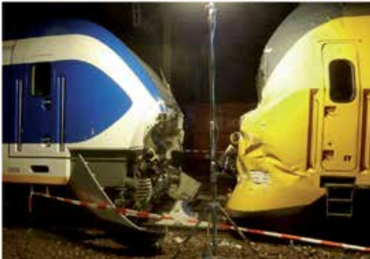
Figure 3: Damage to the sprinter and intercity train at the collision site. Source: Dutch Safety Board.
