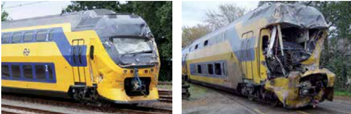
Figure 25: Examples of serious deformations of the driver's compartments of comparable intercity trains (VIRM) as a result of level crossing collisions with a truck; left: Maarheeze, June 2010; right: Wijhe 2005.
