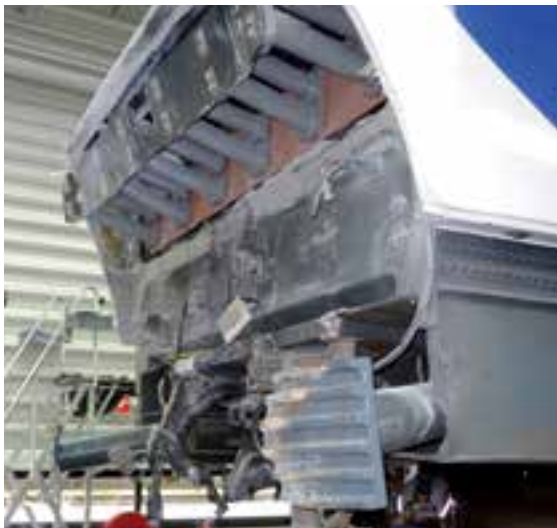
Figure 11a: Top left damaged driver's compartment of the sprinter. Top right: damaged nose of the sprinter. Bottom left: nose of the sprinter following removal of the entire plastic nose. Source: Dutch Safety Board
