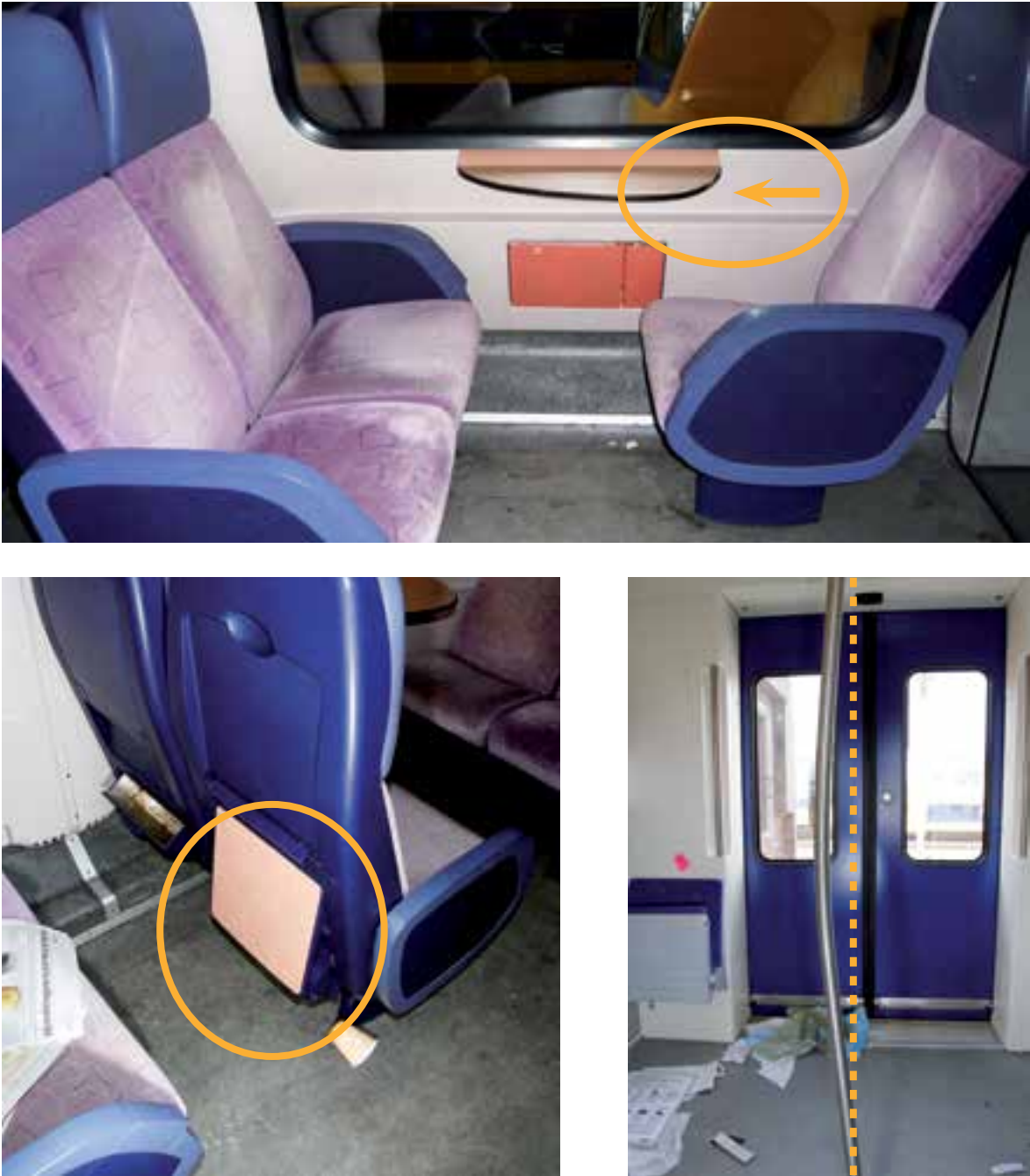
Figure 20: Top: the undamaged table in the section of the intercity where the passenger was fatally wounded; Bottom left: a folded table in the rear of an intercity seat; Bottom right: a deformed bar in the sprinter vestibule, probably bent in a collision with a passenger. Source: Dutch Safety Board
