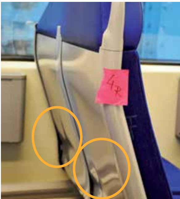
Figure 19: Damage to the intercity and sprinter interiors. Top left: broken plastic in the rear of intercity seats, at head height; Top right: broken plastic in the rear of intercity seats, at knee height; Bottom left: damage to the rear of sprinter seats positioned behind one another in rows. Source: Dutch Safety Board
