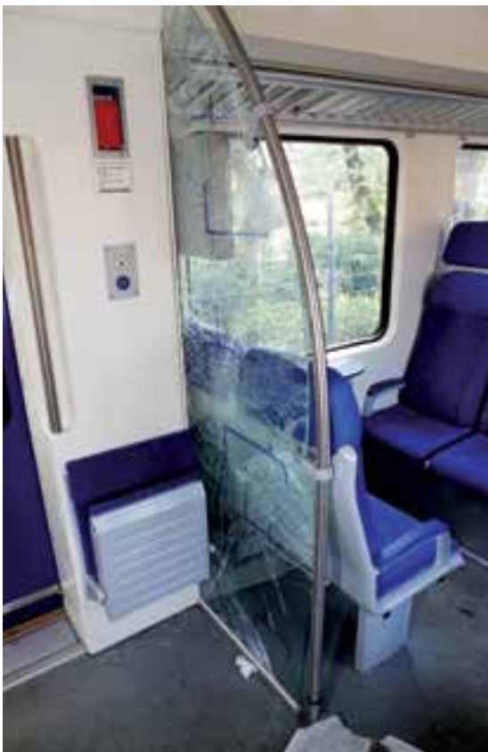
Figure 11b: Top left: broken track fastening. Top Right: deformed handrail. Bottom left: glass wall. Bottom right: deformed seats. Source: Dutch Safety Board
