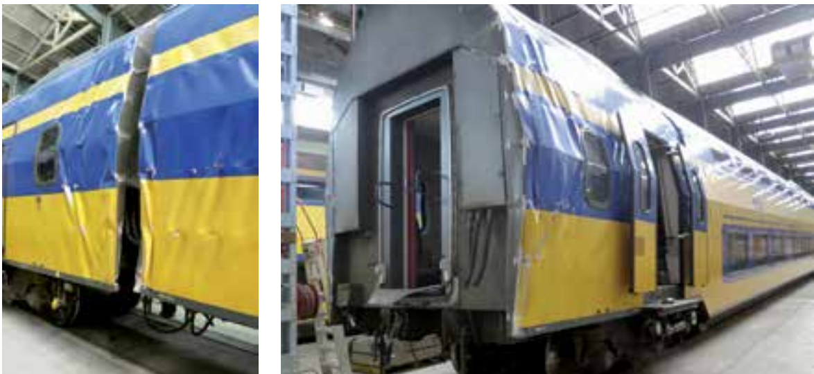
Figure 4: Damage to the intercity coaches. Source: Dutch Safety Board.
