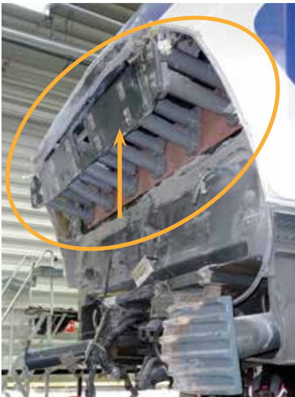
Figure 14: The two photos show the sprinter's twisted crash absorbers (lower photo: after removal of entire plastic nose). Source: Dutch Safety Board
