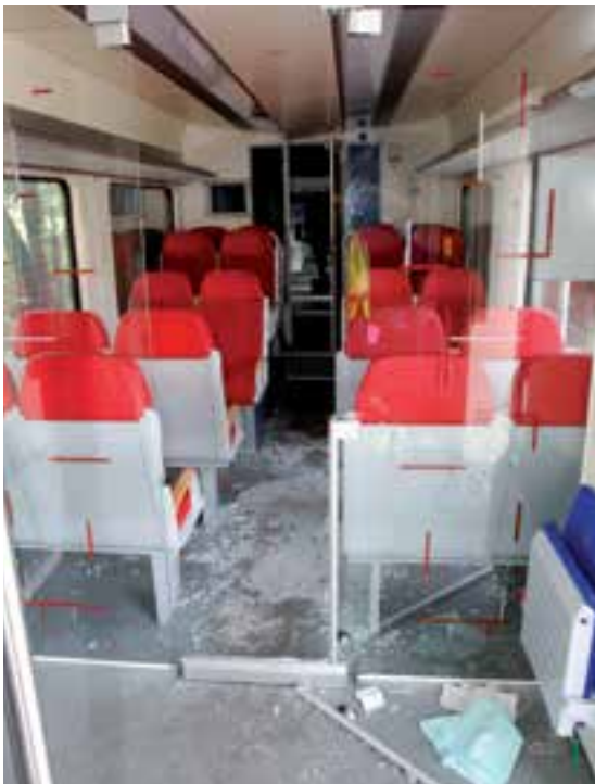
Figure 21: Glass damage. Top left: entrance to intercity passenger compartment; Top right: broken glass partition wall in sprinter; Bottom left: shattered glass door in sprinter; Bottom right: broken and dislodged glass shards in sprinter. Source: Dutch Safety Board
