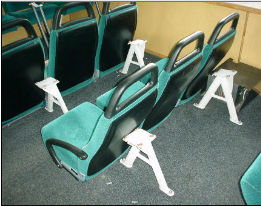
Figure 6: Photo of broken mountings of passenger seats
