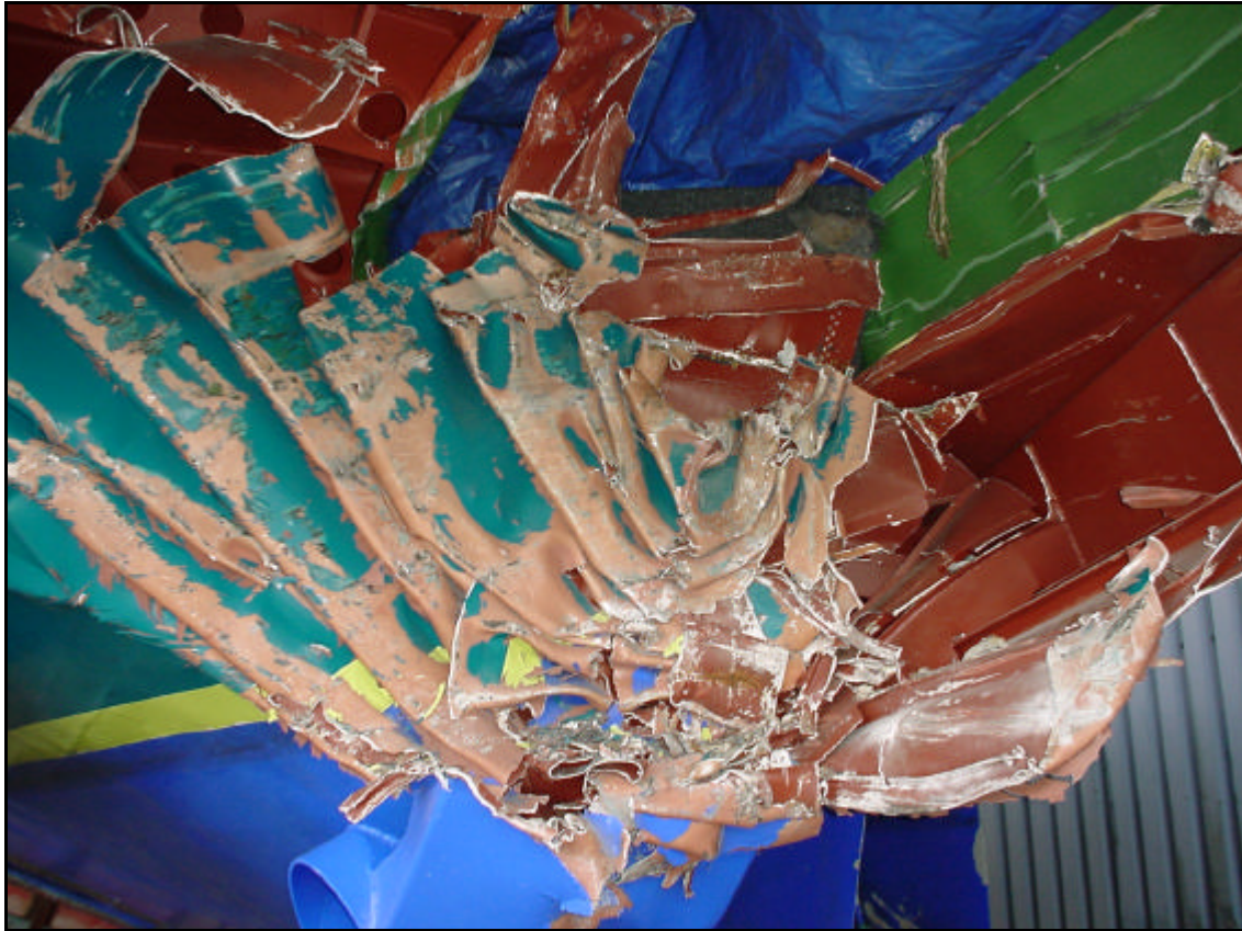
Figure 4: Photo of the deforming of the ship's hull of the Voskhod 605 as a result of the forces exerted at the collision.
