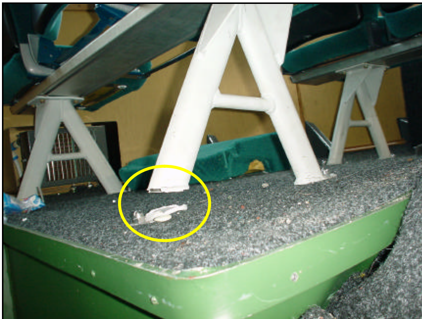
Figure 7: Photo of passenger seat torn off floor mounting.
