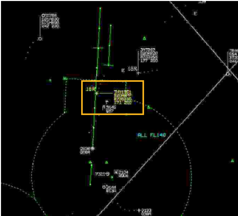
Figure 10: The radar plot on which aircraft TK1951 is still indicated, six miles before the runway.
