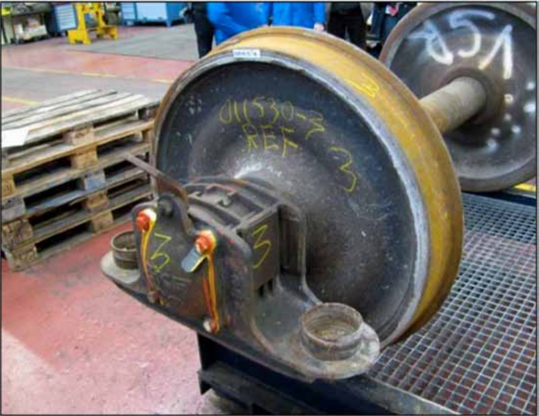
Figure 7: Wheel set with (in the foreground) an axle box.
