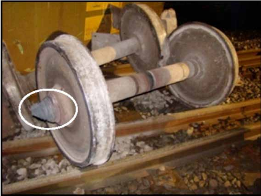
Figure 8: The second wheel set of the eleventh wagon. The left-hand axle journal has broken off/melted.
