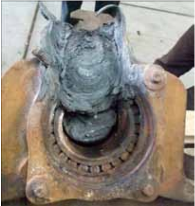
Figure 24: This photo of (the inner side of) the overheated axle box shows that the axle journal erodes its way upwards through the axle box.
