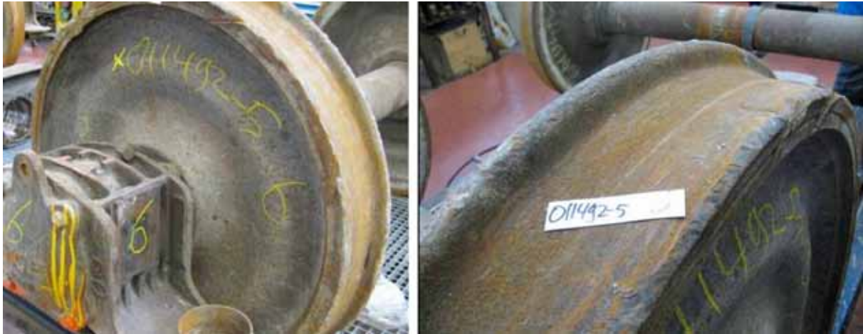
Figure 14: These photos show the damage to the wheels of the front wheel set (of the front bogie of the eleventh wagon) caused by the wheel set running over the concrete sleepers.
