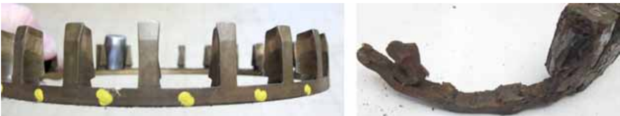
Figure 21: Left: a comb-shaped brass bearing cage of the type used in the relevant bearings. Right: the remains of one of the two bearing cages from the outer bearing mounted in the overheated axle box (with the cage lips broken off).
