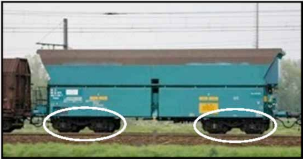
Figure 6: Wagon with two bogies (each of which has two wheel sets).
