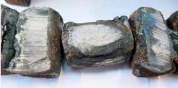
Figure 20: Three rollers from the outer layer: one roller had turned through 90 degrees and flats had worn on all three rollers.
