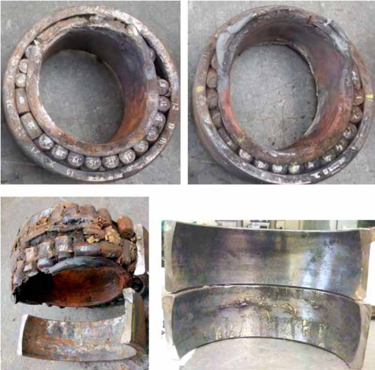
Figure 19: The outer layer from the overheated axle box. the top left photo shows the outer side, the top right photo the inner side. The bottom left photo was taken once the outer ring had been cut through and partly removed. The bottom right photo shows the raceway of the outer ring after the ring had been cleaned.
