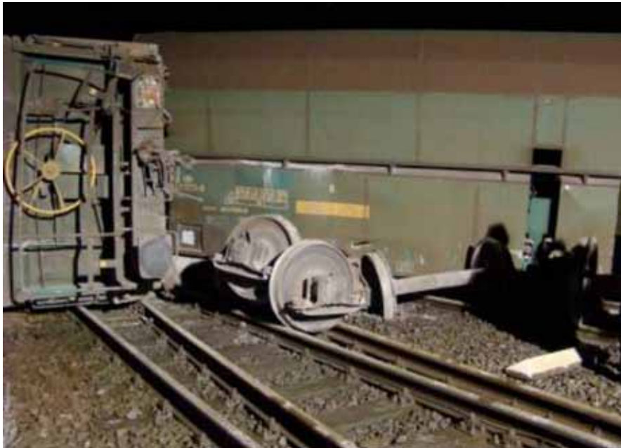
Figure 16: This photo shows some of the derailed wagons and a number of wheel sets that had broken off.
