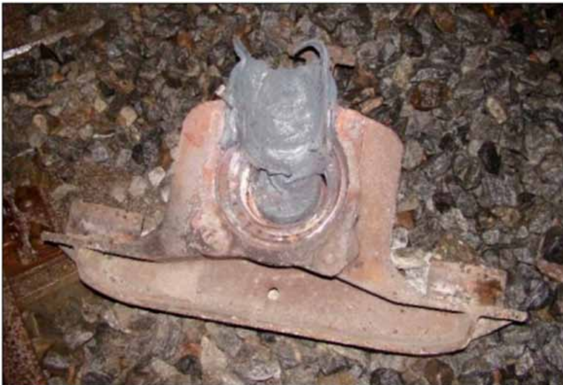
Figure 9: the overheated axle box found next to the track at the location of the derailment.
