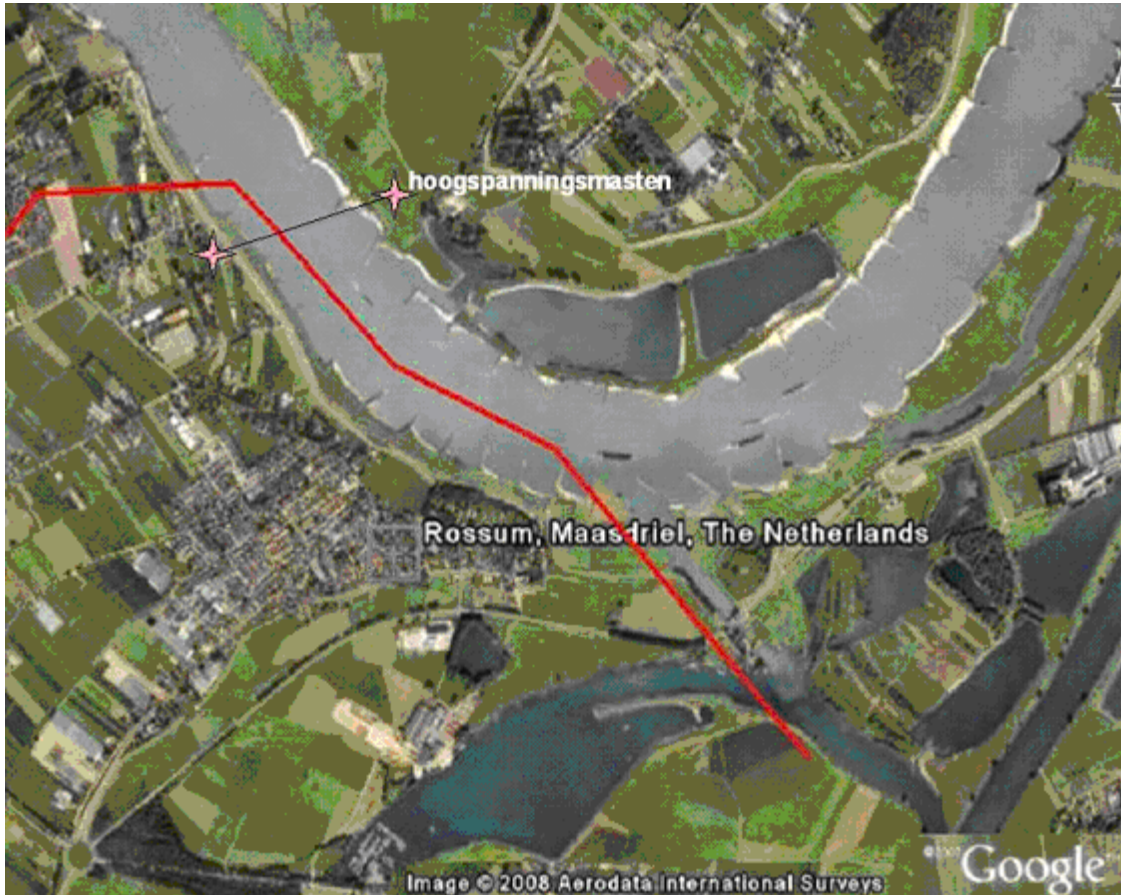
Figure 5: flight path immediately before and immediately after the collision with the power lines
