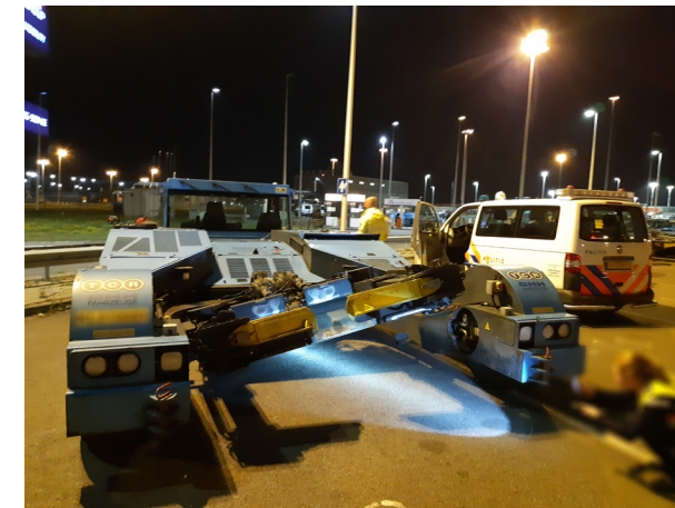
The damaged pushback tug. (Source: Dutch aviation police)
