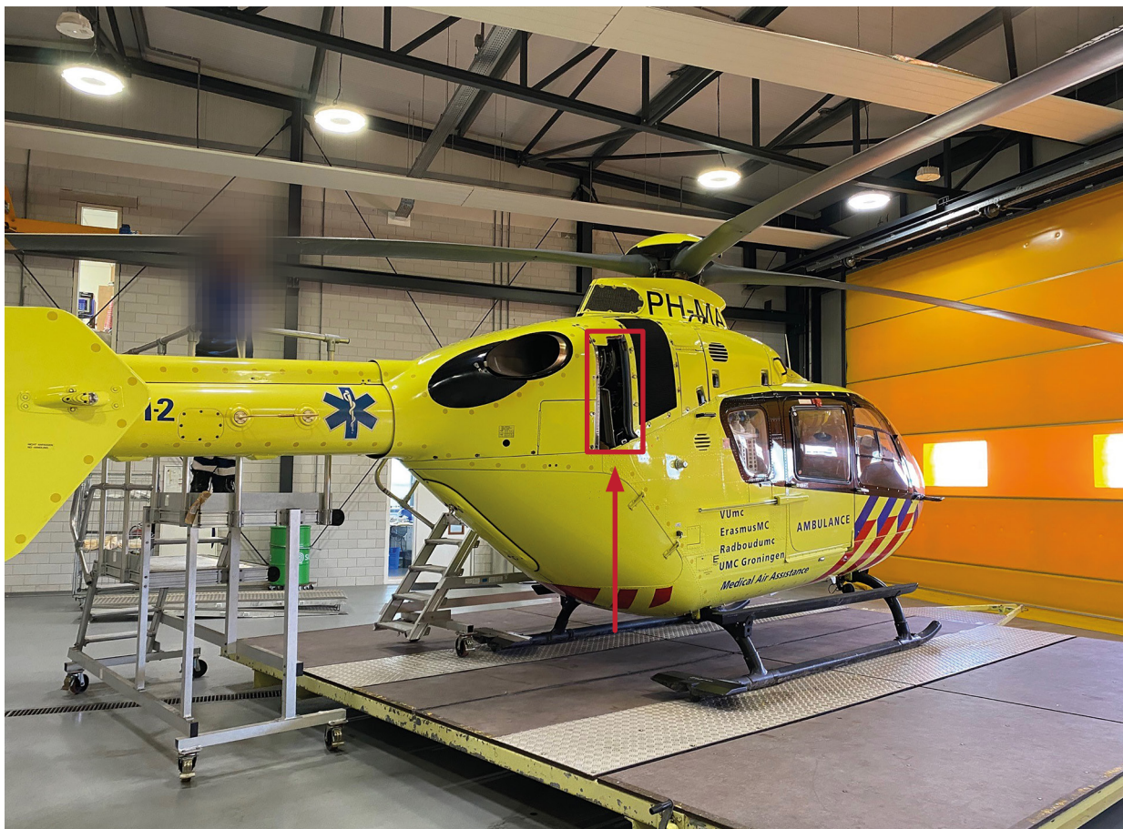
The helicopter with the lost engine inspection panel. (Source: ANWB MAA)
