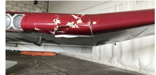
Damage to the left wing. (Source: Dutch Aviation Police)
