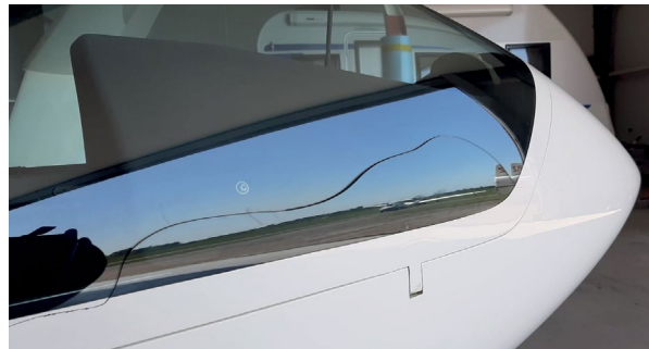
The damaged canopy of the Discus bT. (Source: Pilot)
