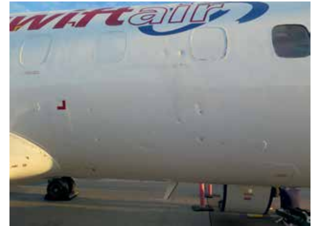
The damaged fuselage of the Embraer EMB-120ER. (Source: AAIB)
