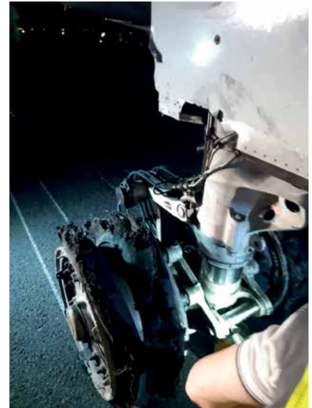
Damage to the landing gear. (Source: ANSV)
