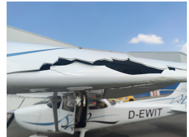
Damage to the left wing. (Source: Airport Operations, Rotterdam The Hague Airport)
