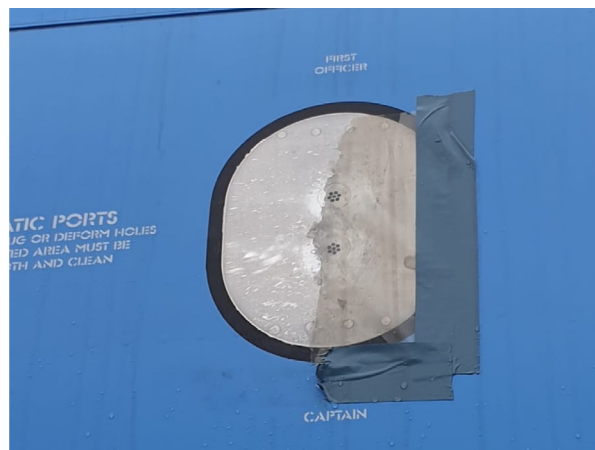
OO-JAV's right hand side captain's and first officer's pitot static port and remnant of used plastic and tape. (Source: Operator of the aircraft)
