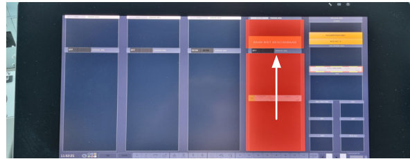
Part of a workstation at Schiphol control tower: the EFS of LVNL. In the above example, runway 18L/36R is unavailable. The red rectangular block (marked with an arrow) contains the tekst 'runway unavailable'. (Source: LVNL)
