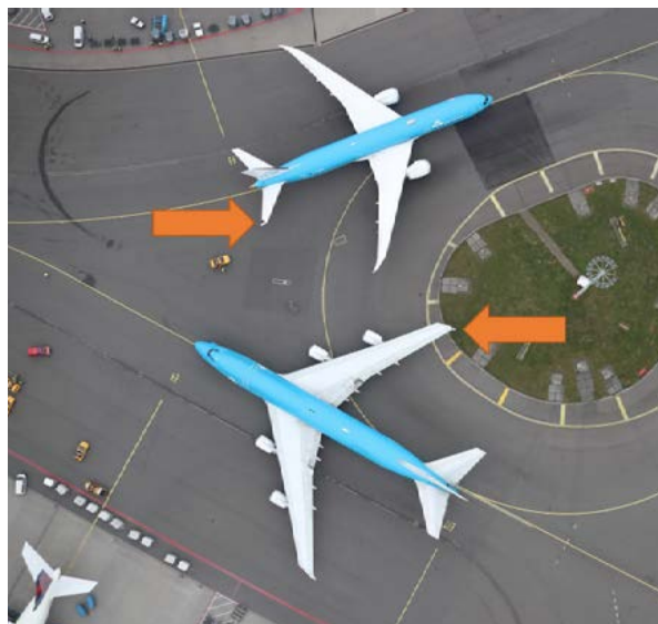
Top view of the position of the aircraft after the accident. The arrows indicate the damaged aircraft parts. (Source: Dutch aviation police)
