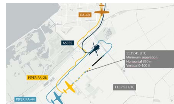
Both aircraft on final and the airprox. (Source of data: LVNL)
