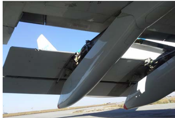
The right wing trailing edge inboard flap system and damage. (Source: owner of the aircraft)
