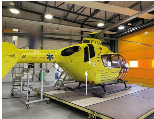
The helicopter with the missing engine inspection panel. (Source: ANWB MAA)
