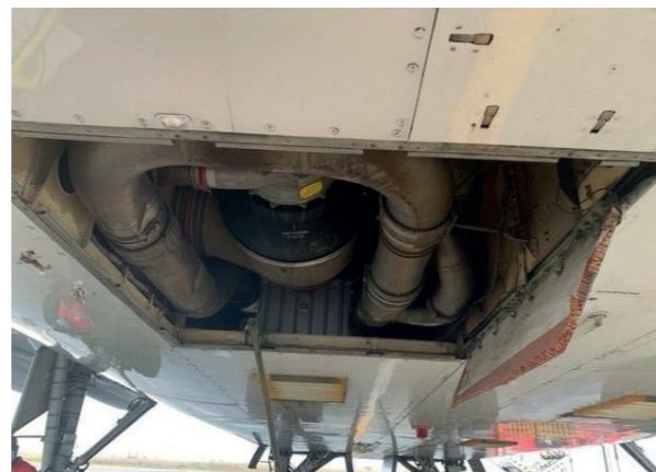
The location of the lost panel.
