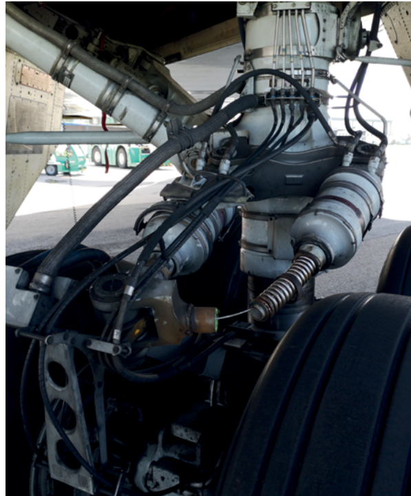
Right main landing gear. (Source: JIAAC)
