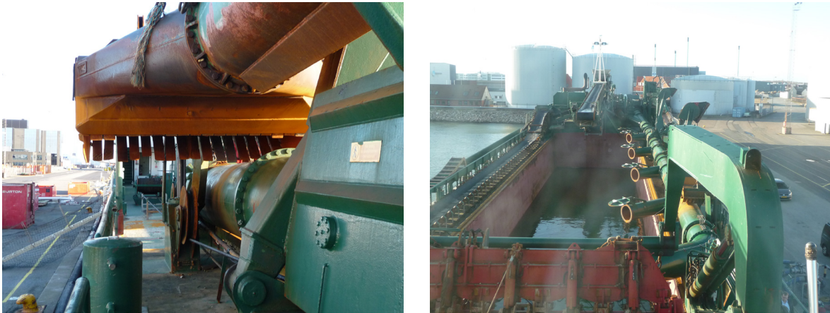
Figure 3: Suction head (left) and cargo hold with loading pipe (right).
