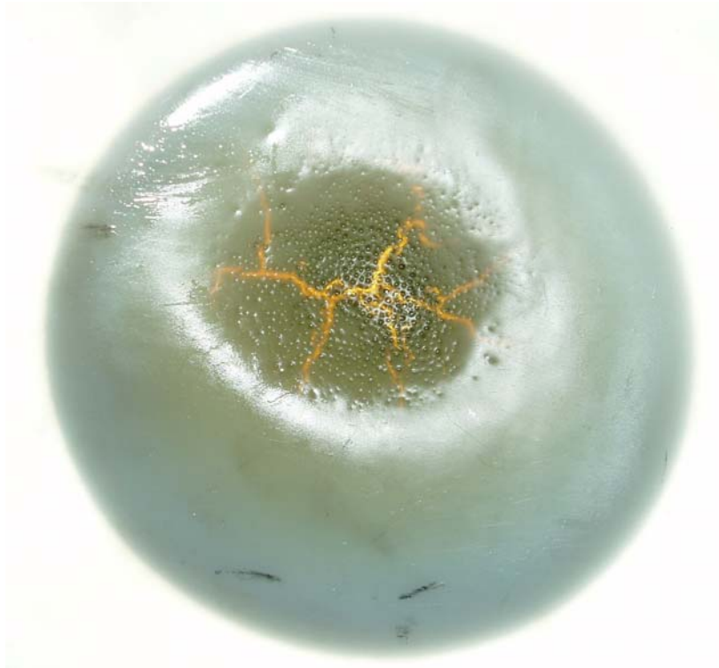
Figure 22a: HDPE panel after water test (view from liquid side). The failure mechanism is pitting to produce holes a few hundred micron across. The characteristic leakage rate is of order 1 g/s
