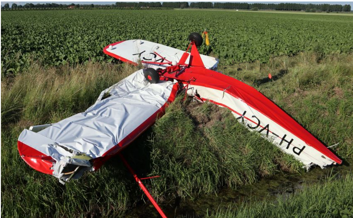
Figure 4: Wreckage of PH-VCY, damaged right wing (lower left corner) and the cut-off angle rear fuselage. (Source: Dutch Safety Board)
