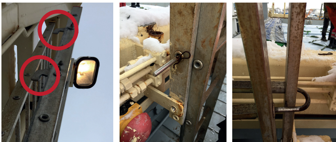
Figure 5: Hooks and securing mechanism for the adjustable ladder. (Source: Dutch Safety Board)
