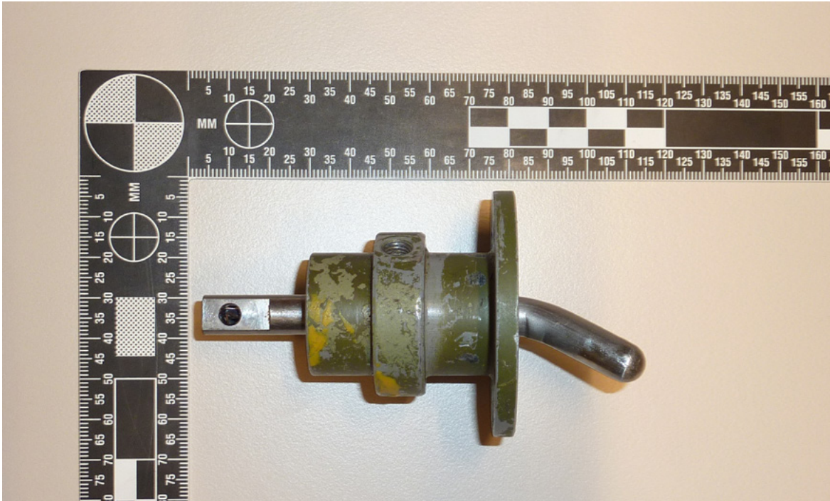
Figure 6: Bent left hand lock pin. (Source: Dutch Safety Board)
