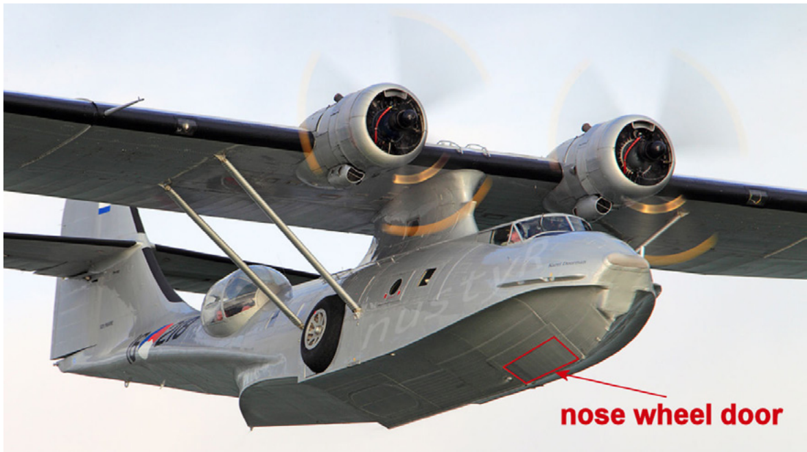
Figure 4: Nose wheel doors closed. (Source: nustyR)
