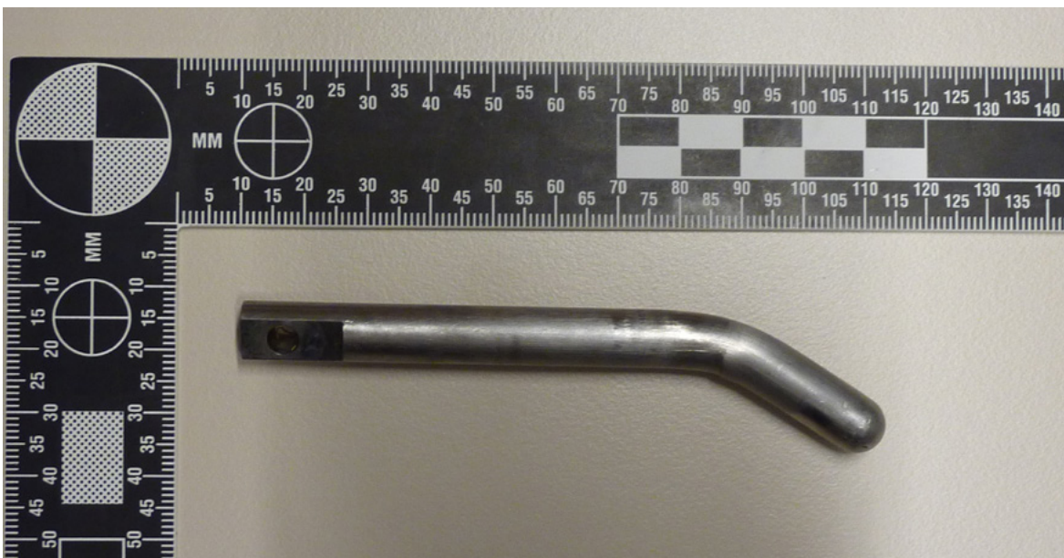
Figure 7: Disassembled left-hand lock pin. (Source: Dutch Safety Board)
