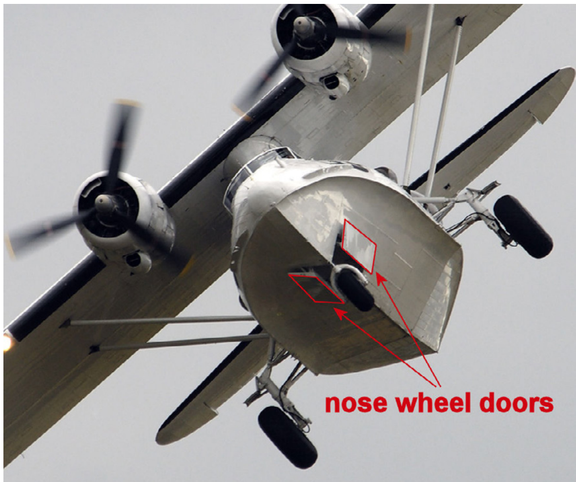
Figure 3: Nose wheel doors open. (Source: Airplane-Pictures.net / Alistair Bridges)
