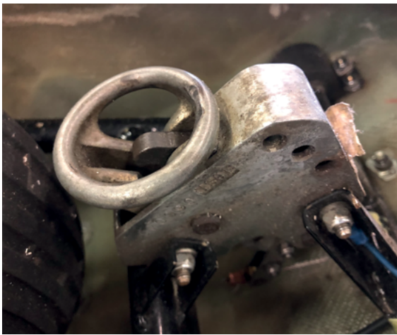
Figure 3: The centre of gravity release hook of PH-1150. (Source: Dutch Safety Board)
