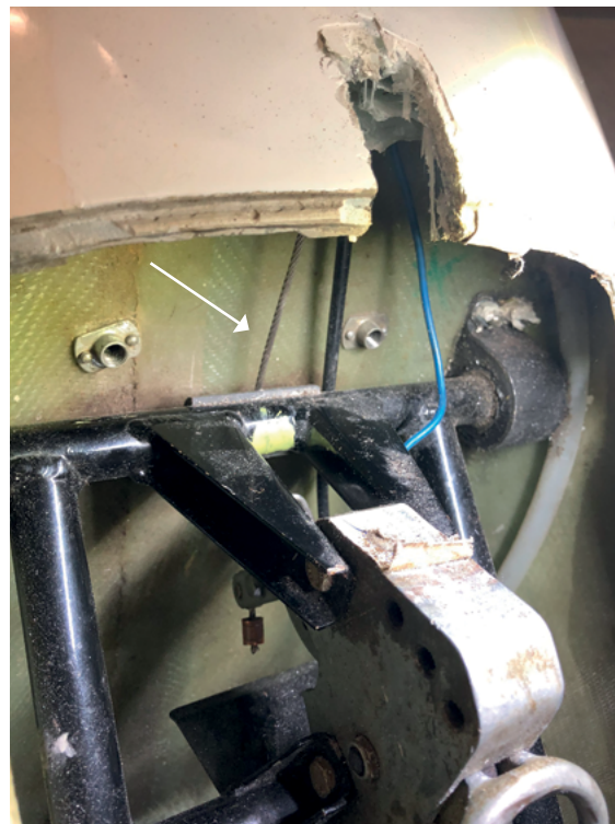
Figure 7: The metal cable of the release mechanism after the routing adjustment. (Source: Dutch Safety Board)
