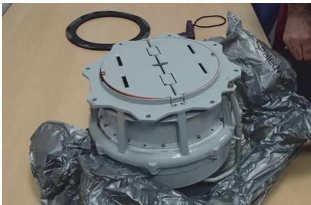
Defecte positive pressure relief valve (PPRV). (Foto: AAIB)
