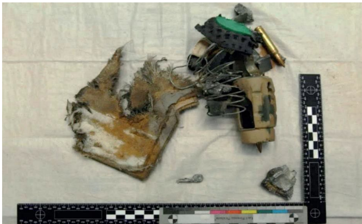
Figure 6: Content of the paper bag: visible are fragments of a shock pylon, a part of a shoe, rounds, a magazine spring, (probably) a cover of the mortar, straps of the transport safety of the grenade and the rubber cover of the sights of a Colt rifle. (Picture: TNO)
