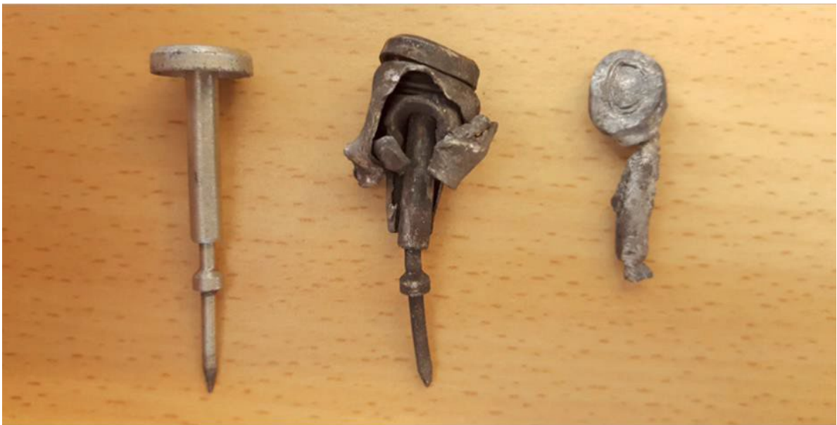
Figure 28: Unused firing pin (left), firing pin from the test in armed position (centre) and from the accident mortar round (right). (Picture TNO)
