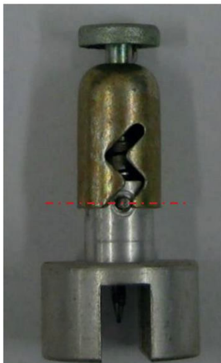
Figure 24: M6-N fuze mechanism composed of correctly positioned zigzag cross-pin at the beginning of the first "knee" of the zigzag slot (Picture: TNO)
