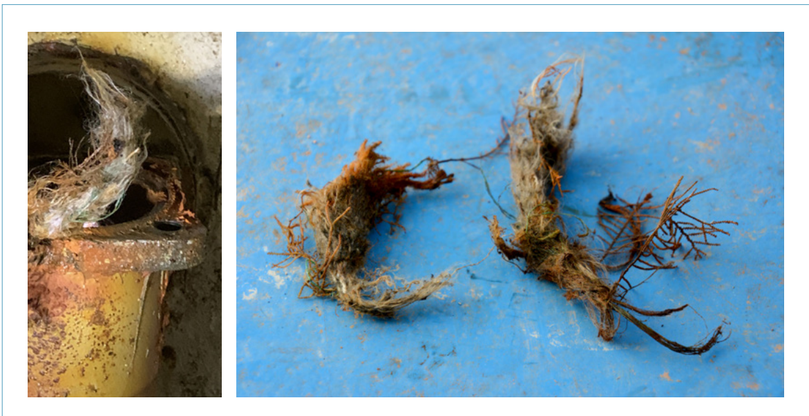
Figure 20: Cordage in the starboard bilge pump outlet. (Source: National Police)
