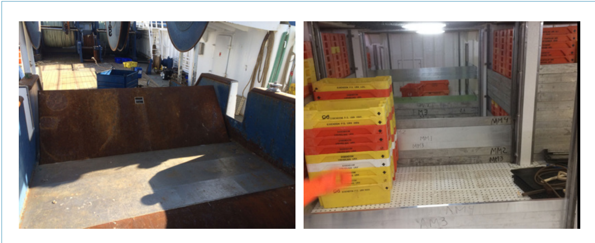
Figure 13: Hydraulic hopper hatch open. (Source: Maaskant Shipyards Stellendam)
