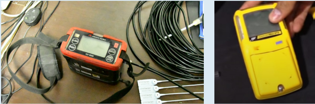
Figure 8: photograph left multi gas meter, photograph right personal combined gas meter.
